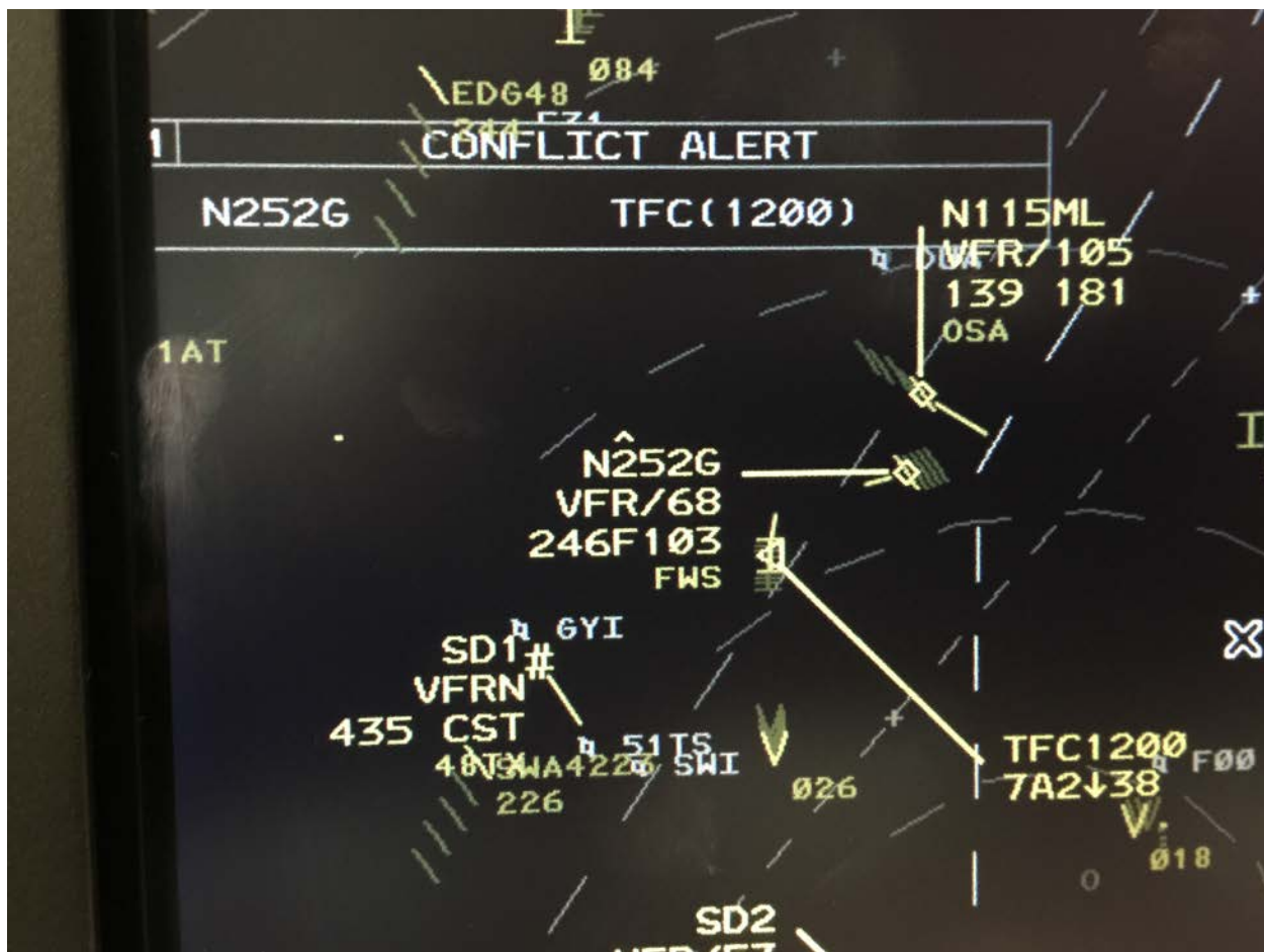
Figure 2 – Position of N252G at 1502:14 after declaring emergency but before being issued vectors.
