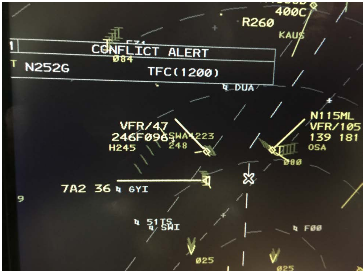
Figure 4 - The radar position of N252G at 1504:18 after pilot requested a closer airport; the aircraft is indicated by the "VFR/47" data tag.
