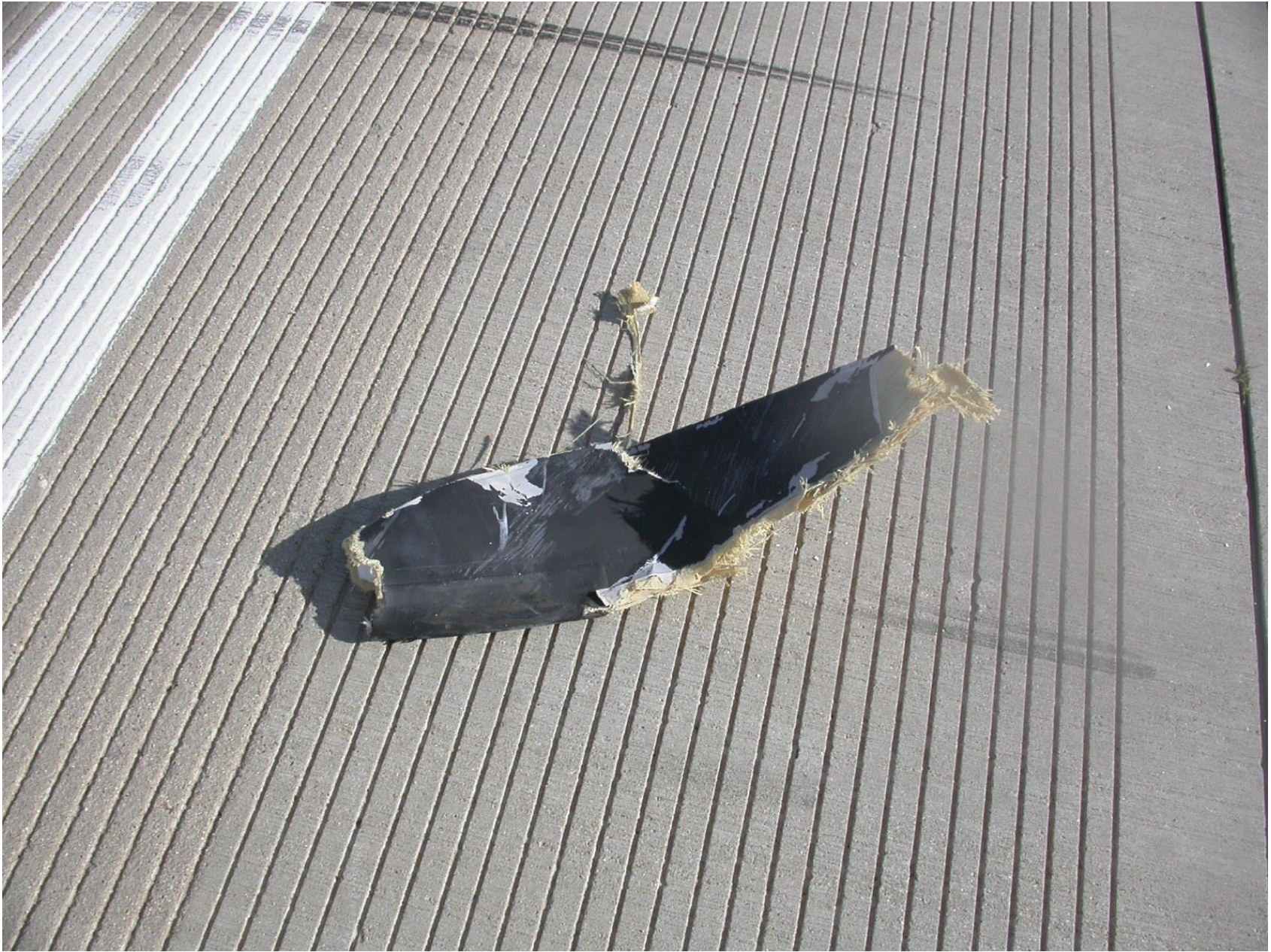
Photo 7 – Broken propeller blade with heavy damage
