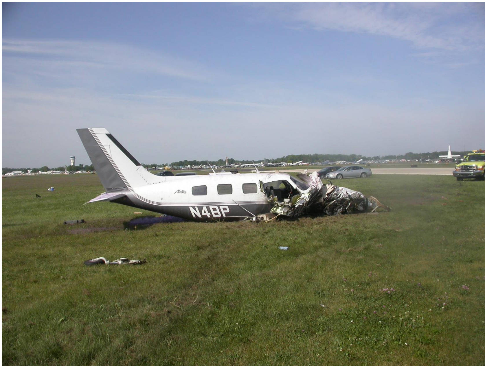
Photo 10 – View of right side of the airplane with the right wing missing
