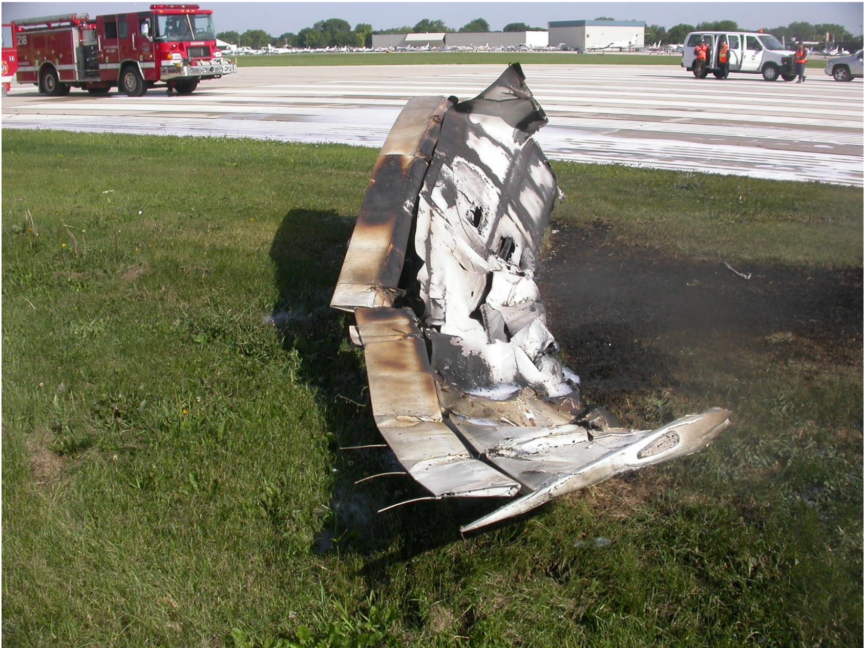
Photo 9 – View of separated right wing with impact and fire damage
