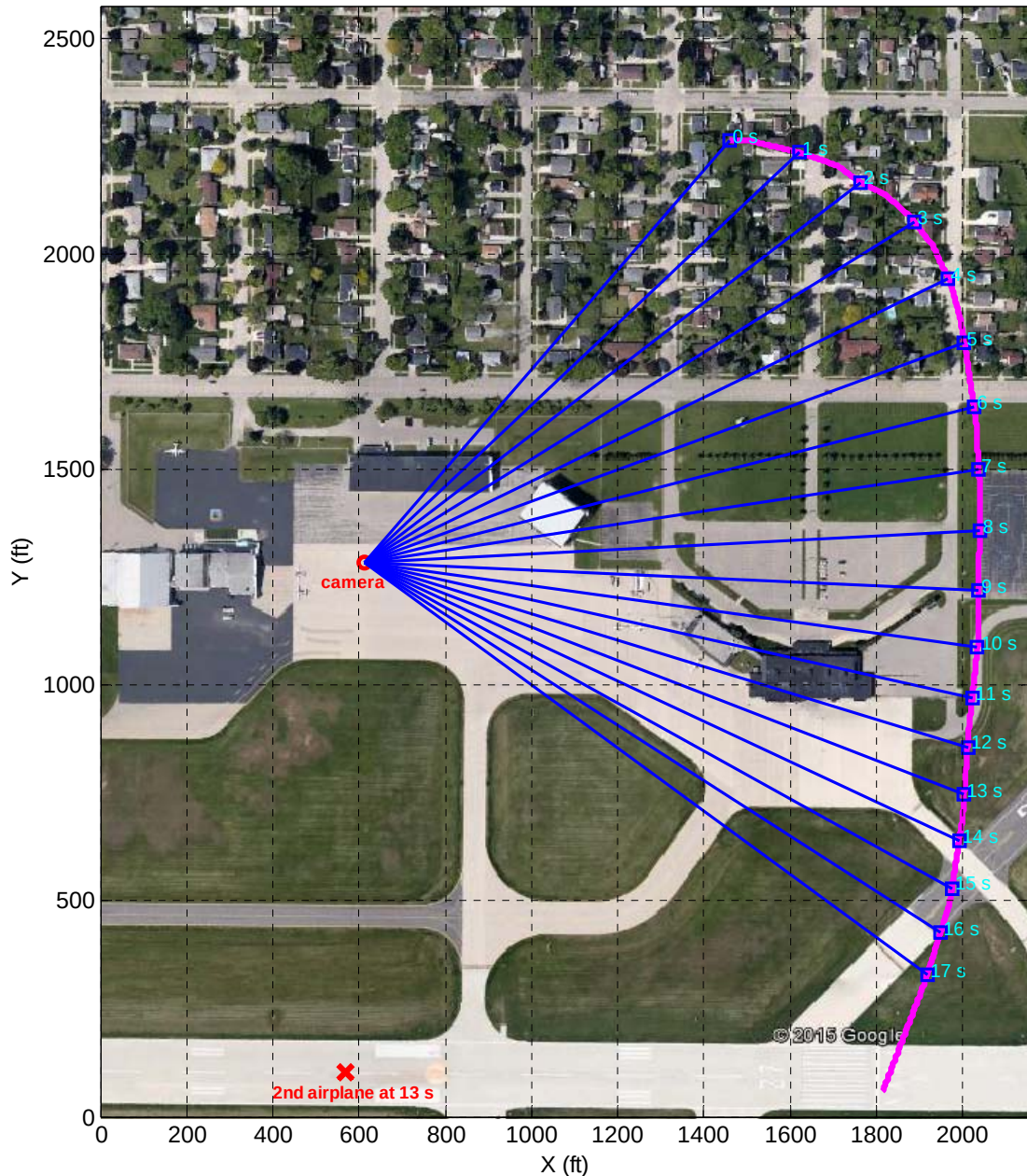
Figure 2 Accident Airplane Ground Track and Eighteen Analyzed Trajectory Points
