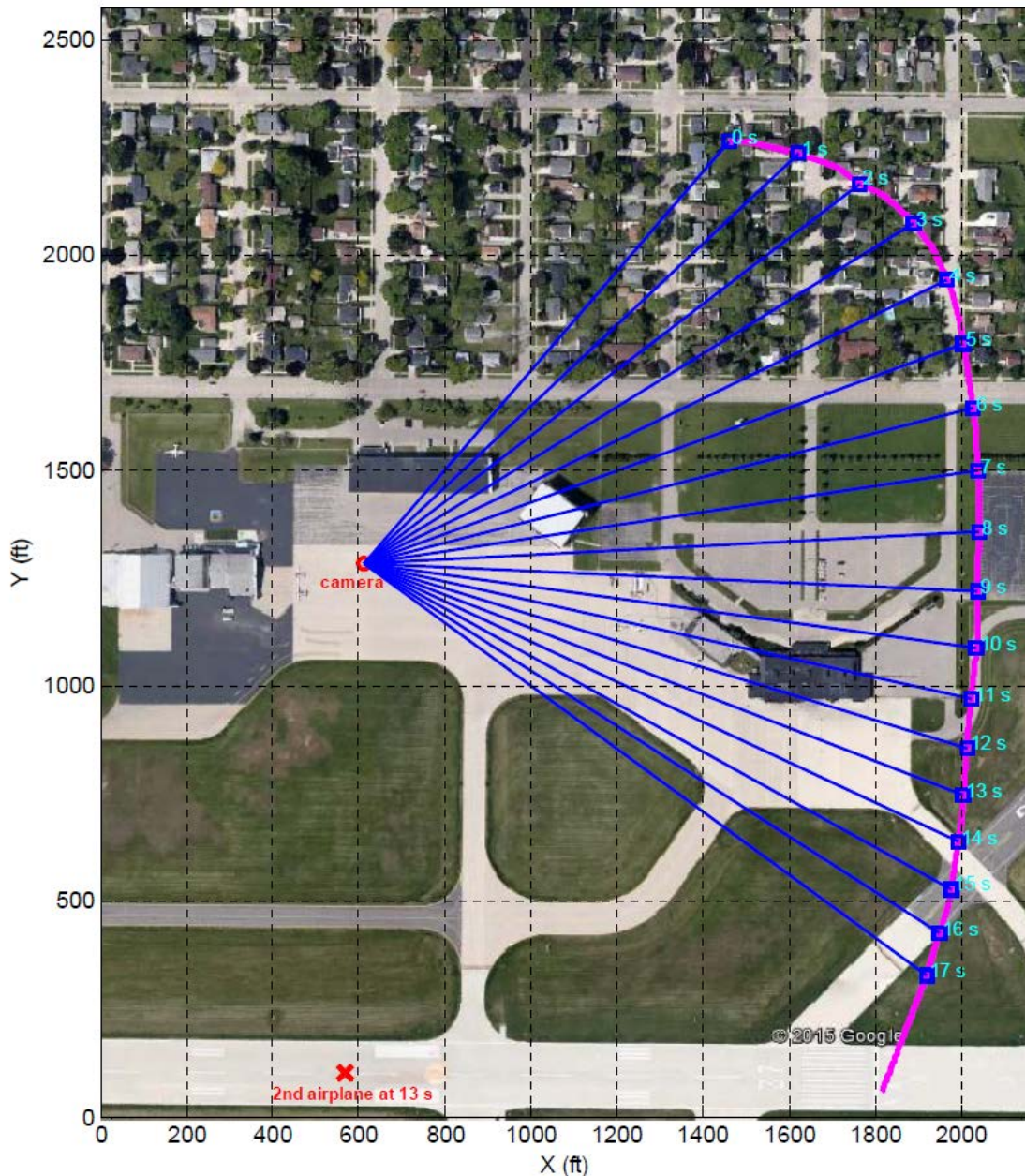
Figure 3: Graphic from video study showing estimated relative positions of N4BP and the preceding runway 27 departure.
