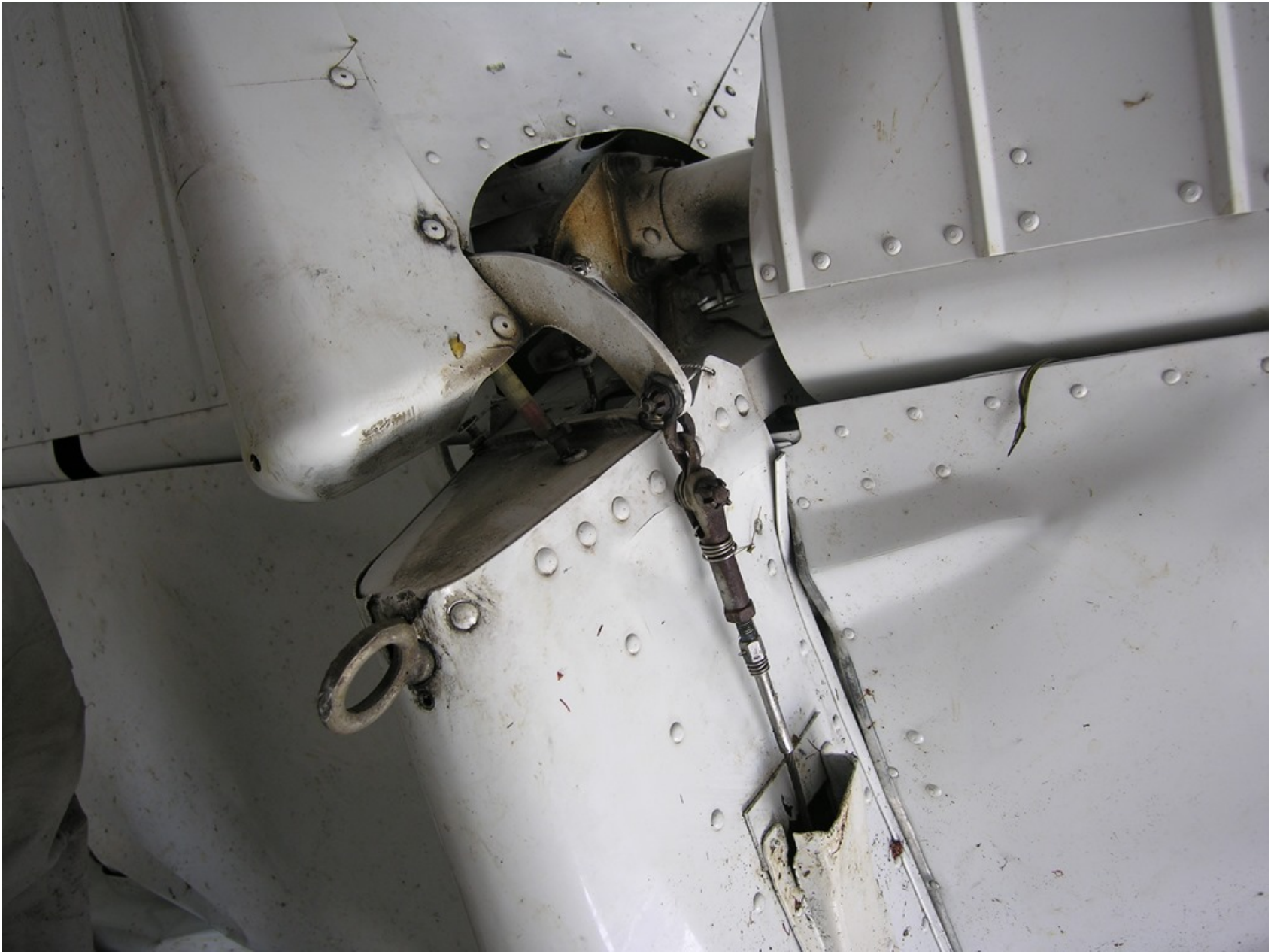
Photo 4 - Rudder cable attachment
