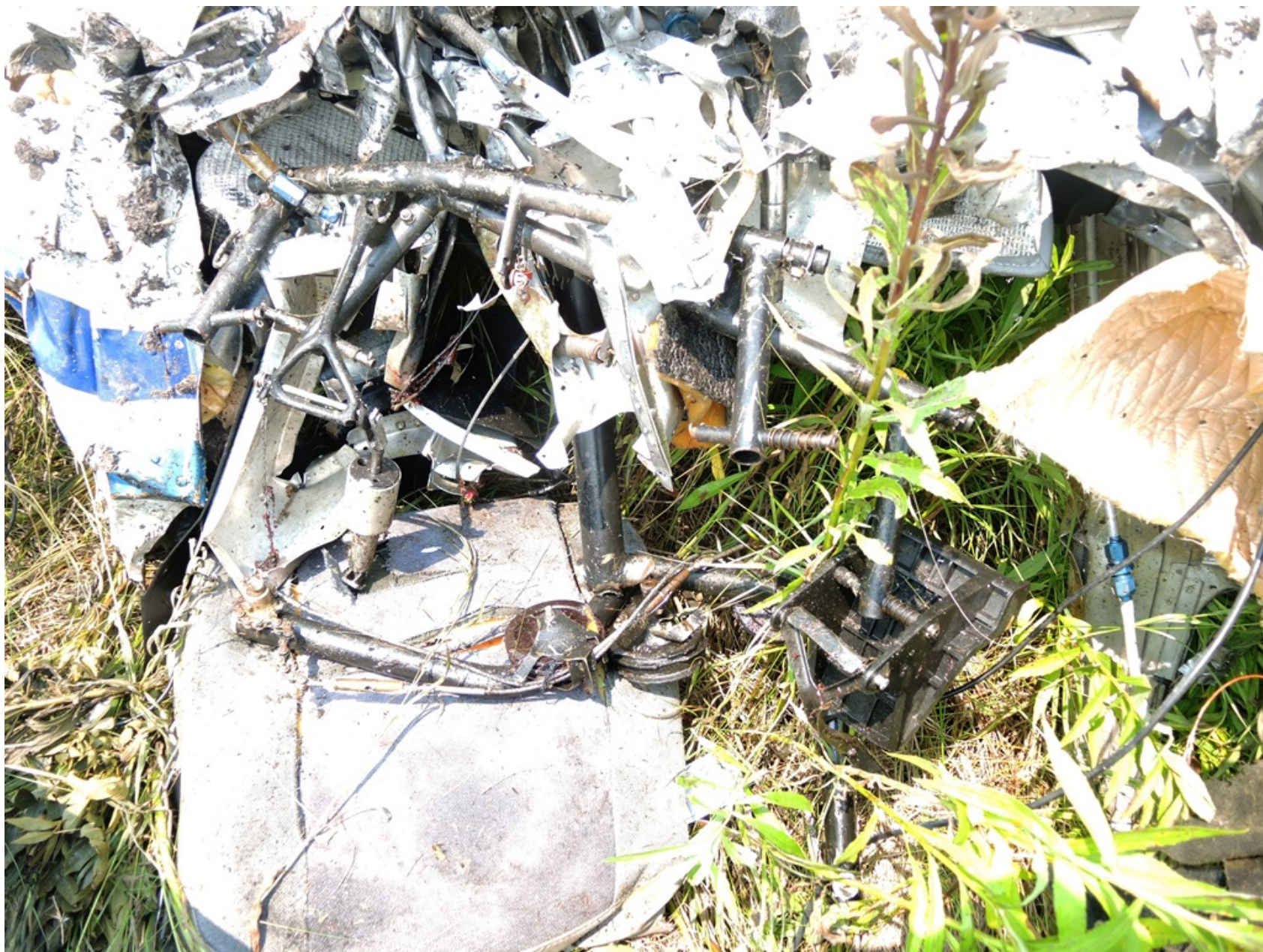
Photo 3 - Wreckage - part of rudder pedals
