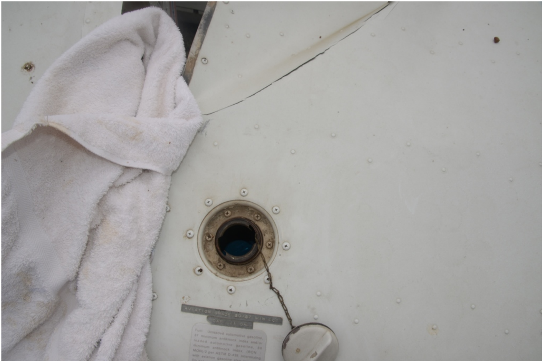
Photo 10 - View of blue liquid below the left fuel tank's filler neck.
