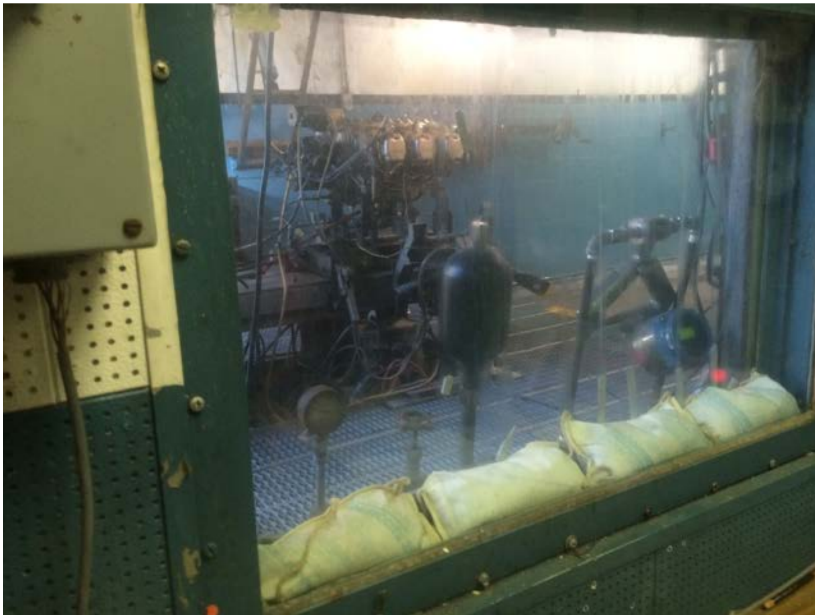
Photo 12 - View of the accident engine operating in a test cell.
