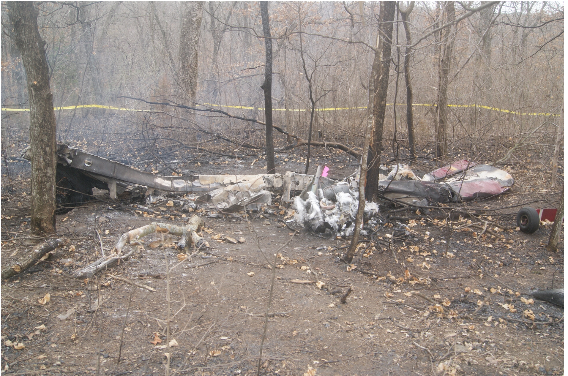
Photo 5 - Inverted wreckage of N623HS, revealing both wings and engine. Note the smoke haze.
