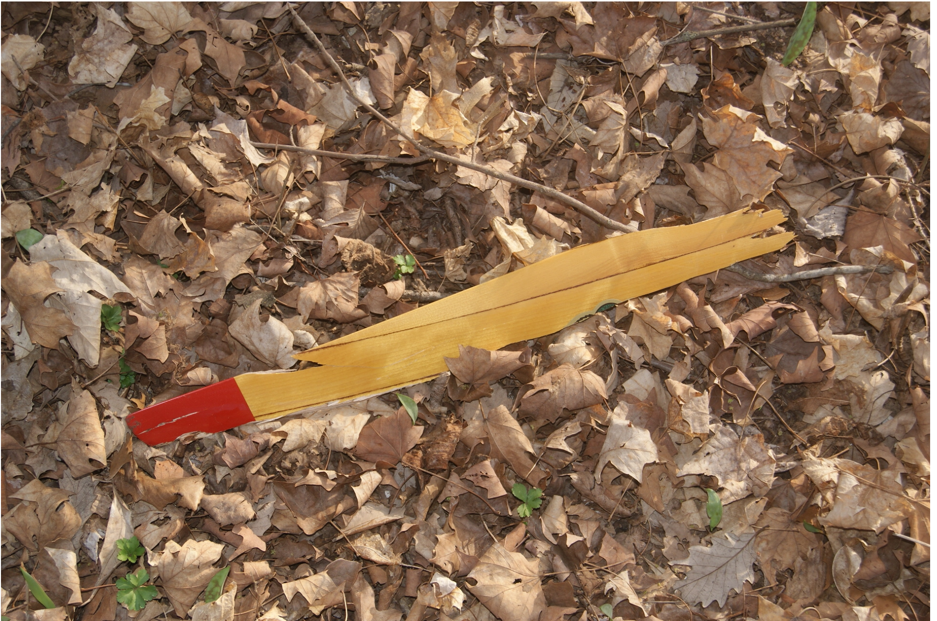
Photo 7 - Substantive portion of propeller blade A.
