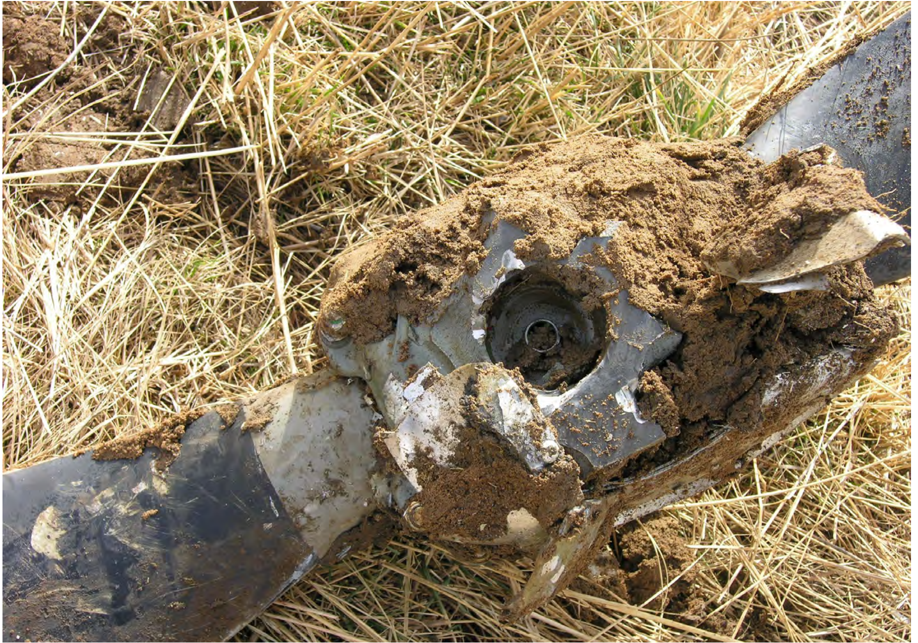
Photo 6 – Propeller – showing fracture surfaces on the propeller flange (NTSB Photo)
