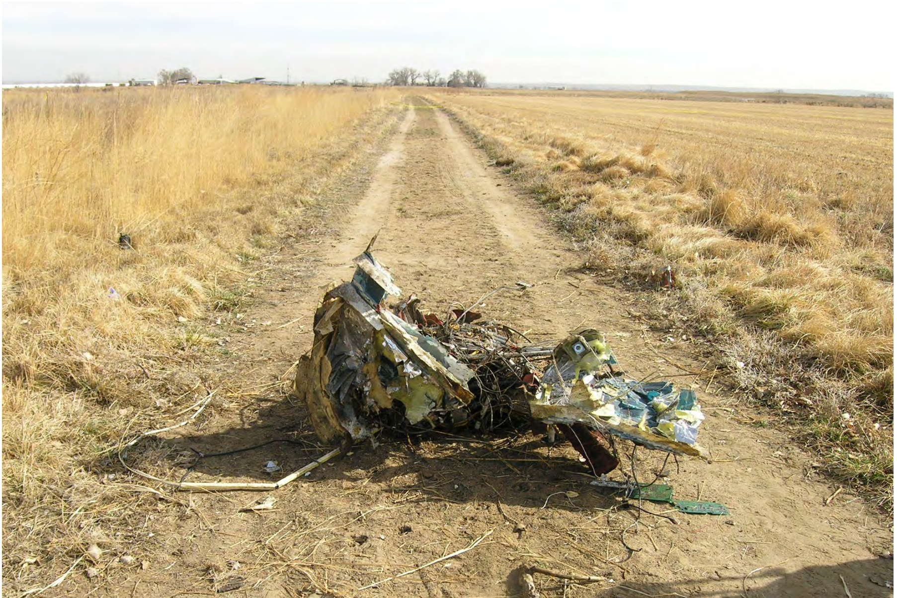
Photo 7 – Completely separated forward fuselage and engine – viewer looking east (NTSB Photo)
