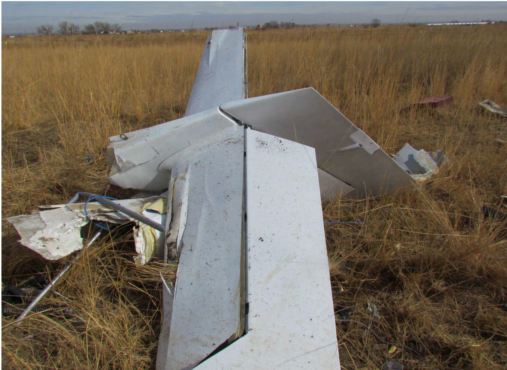
Photo 8 – Completely separated tail surfaces – viewer looking northeast (NTSB Photo)
