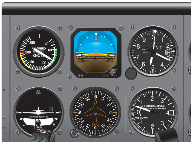
Figure 10-3. Establish a positive climb.
