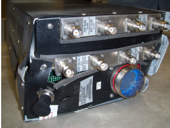
Figure 2: deformation of right portion of main shell
