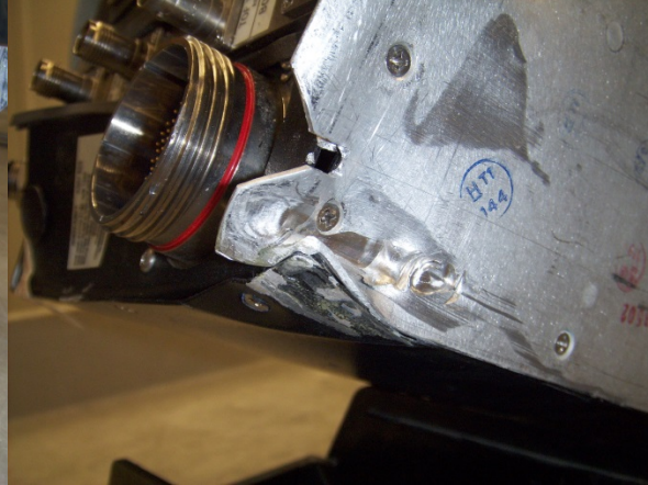
Figure 3: deformation of left portion of main shell
