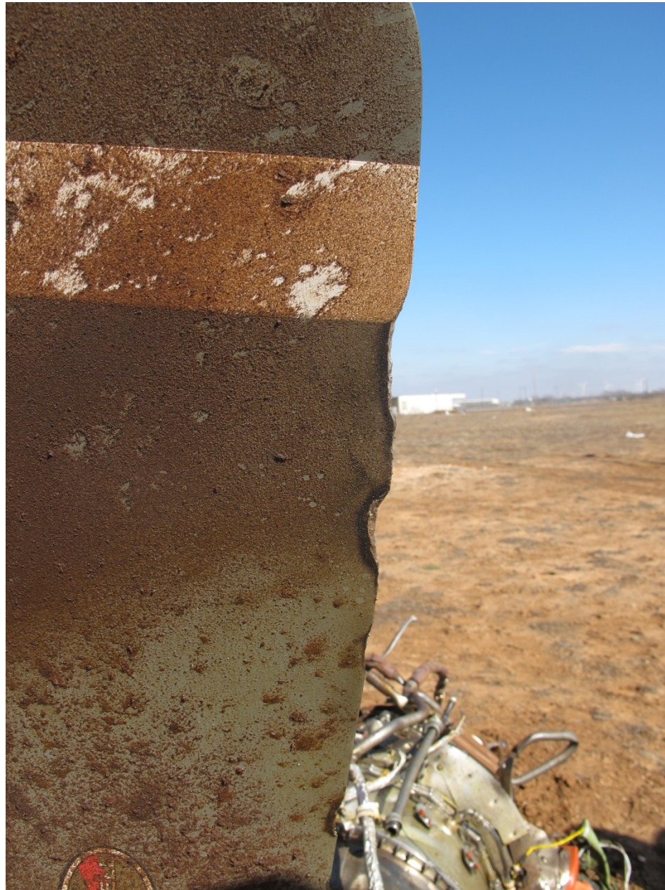
Photo 6 – Propeller blade damage
