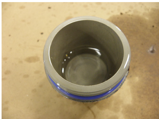
Photo No. 13, Residual fuel in filter bowl
