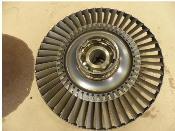
Photo No. 11, 1 st stage power turbine disk
