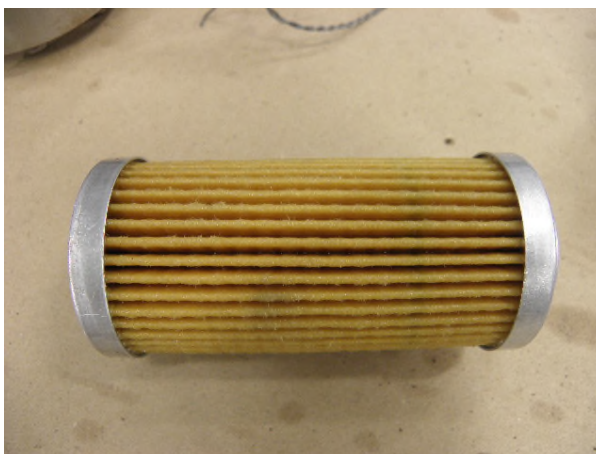
Photo No. 14, Fuel filter
