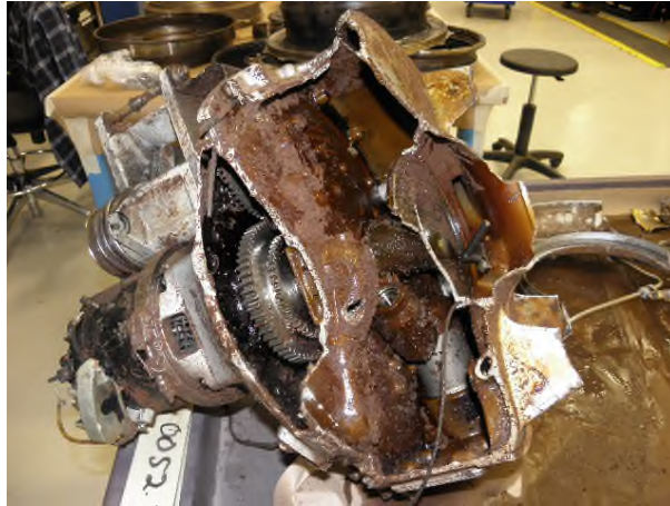
Photo No. 5, Accessory gearbox
