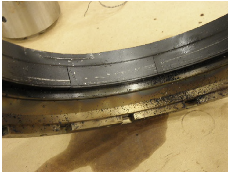
Photo No. 7, Compressor turbine shroud segment rubs
