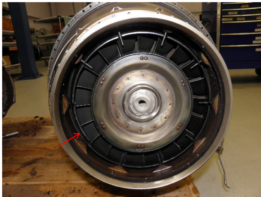
Photo No. 8, 1 st stage power turbine vane and housing
