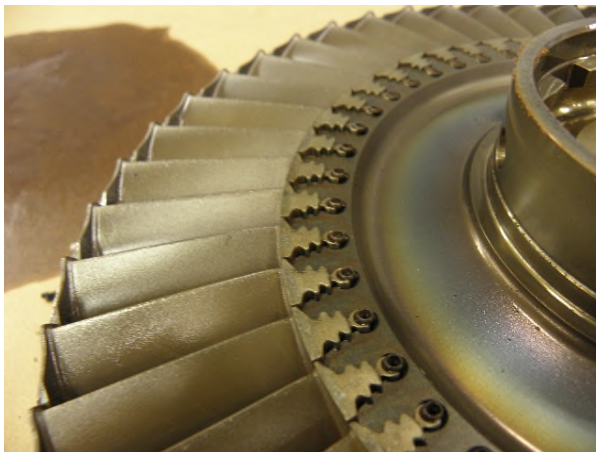
Photo No. 12, 1 st stage power turbine disk
