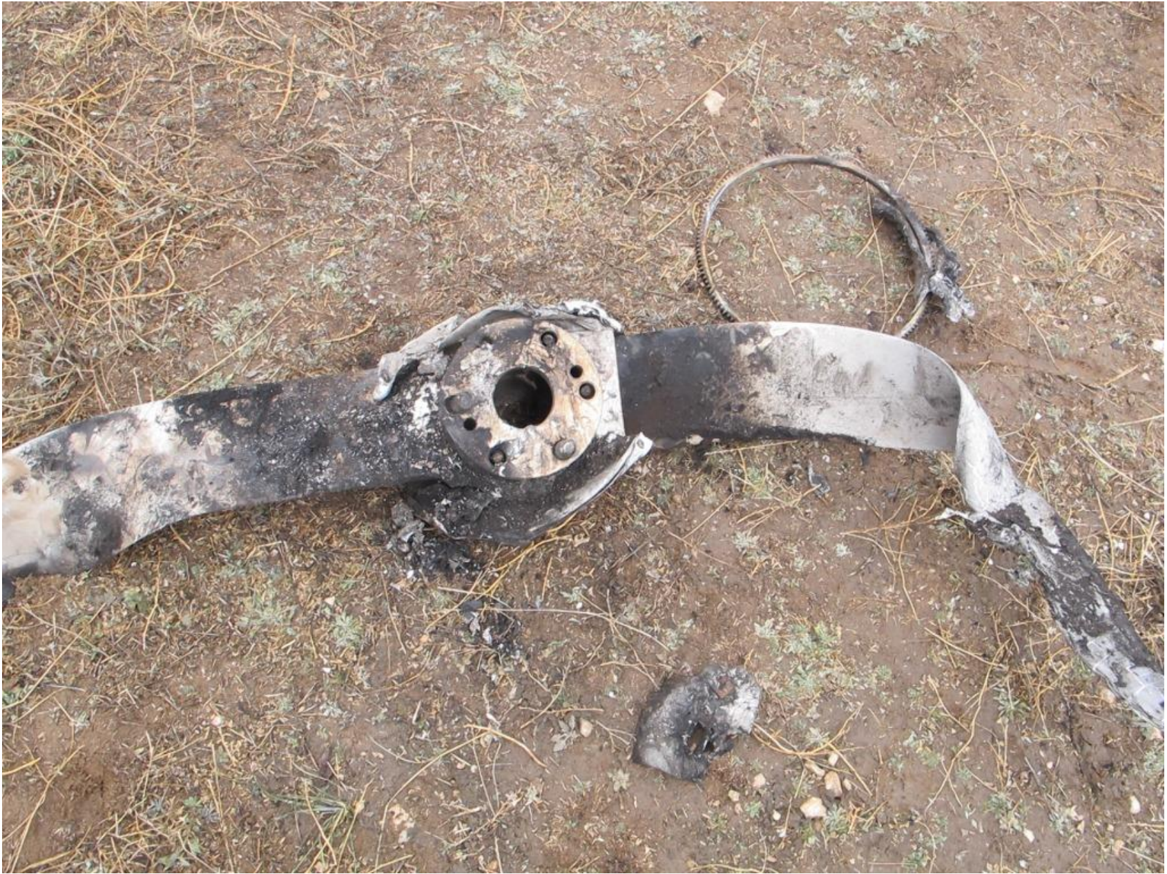
Photo 10 – View of fire damaged propeller
