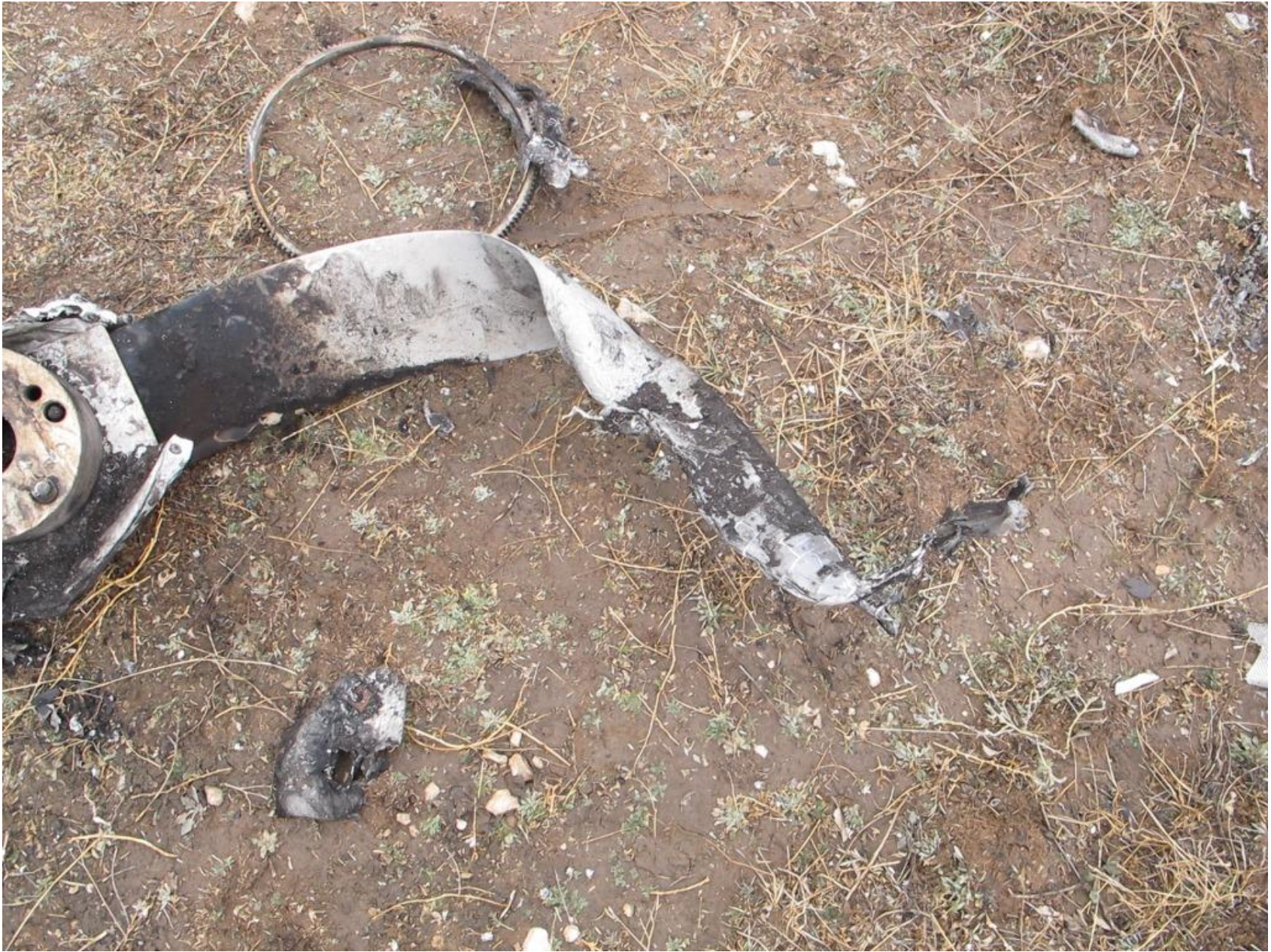
Photo 11 – View of bent and twisted propeller blade
