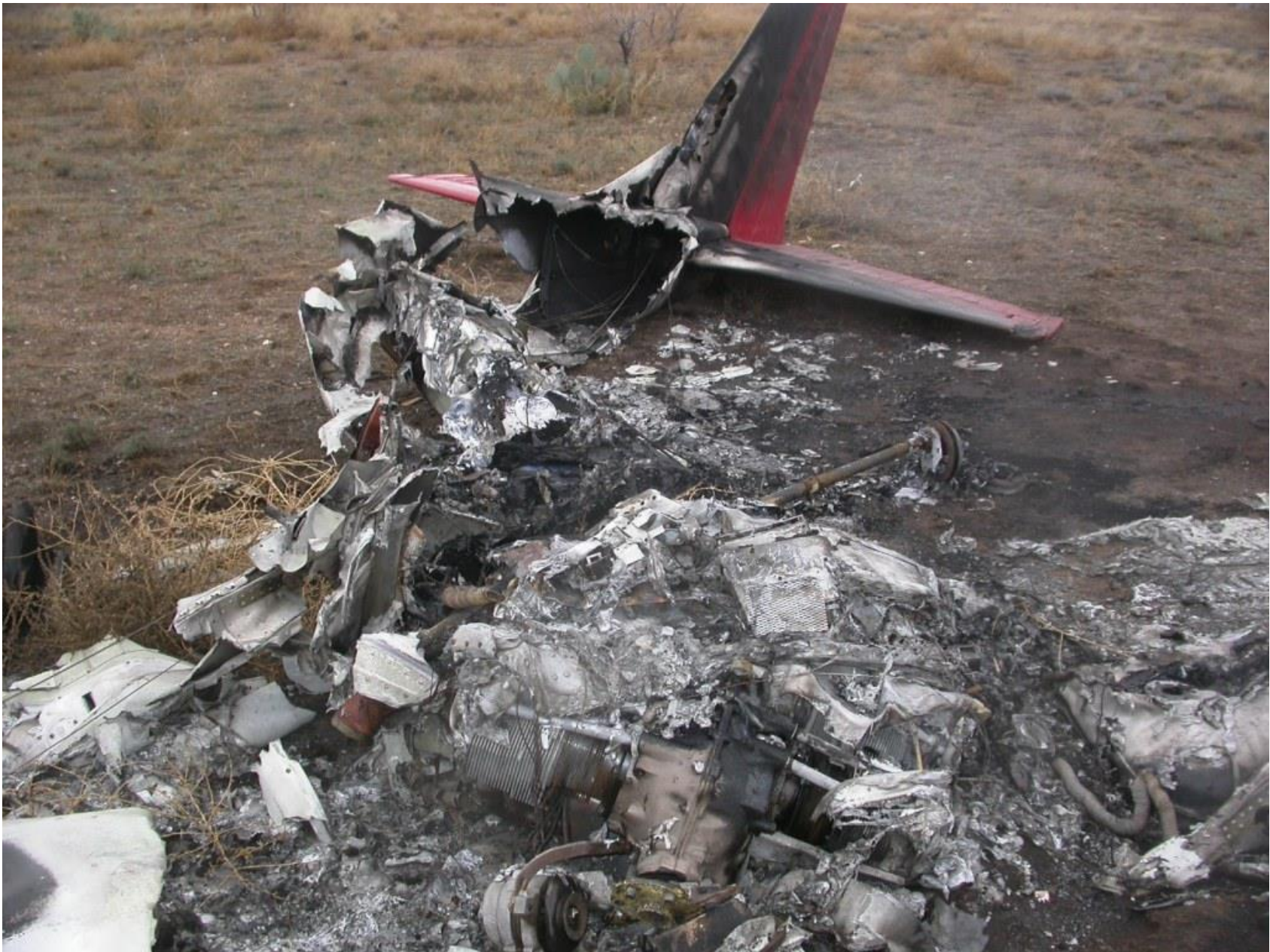
Photo 5 – View of burned engine compartment, cabin, and fuselage
