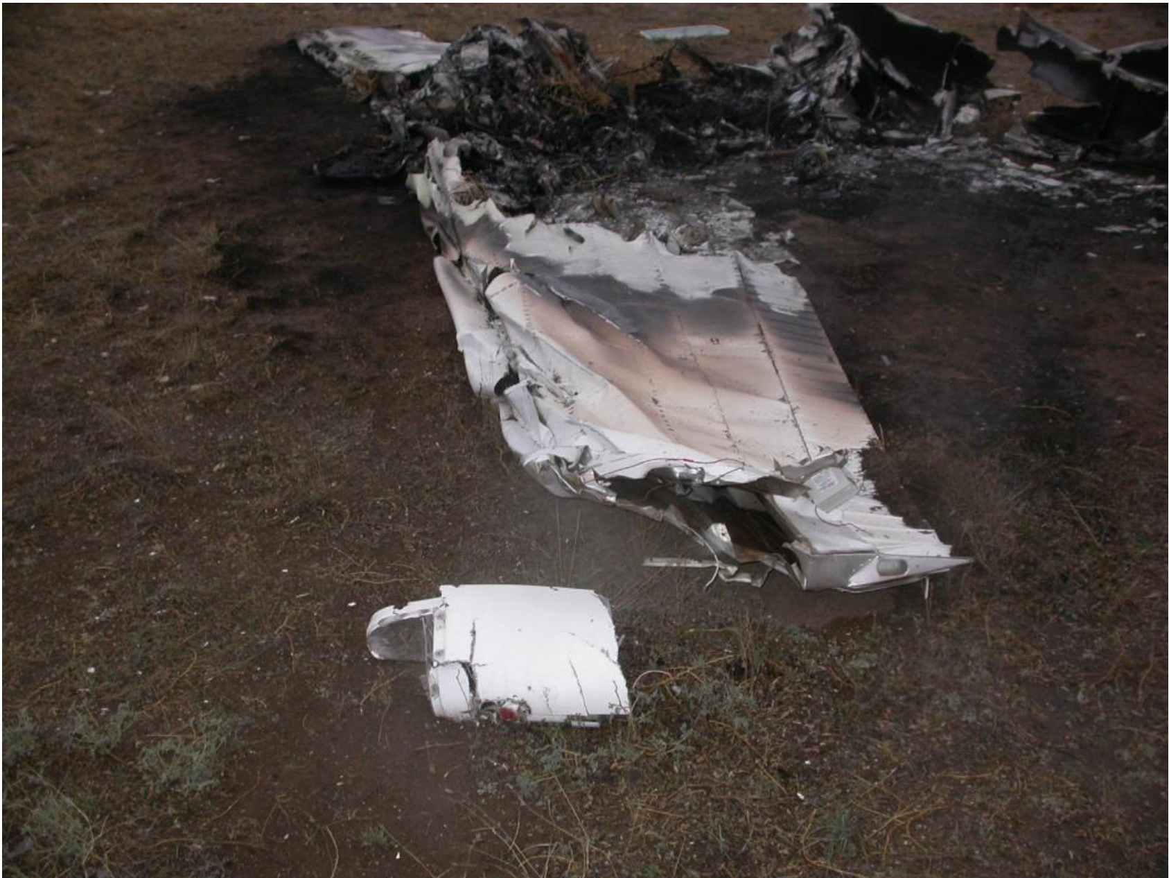
Photo 4 – View of damage to the outboard section of the left wing
