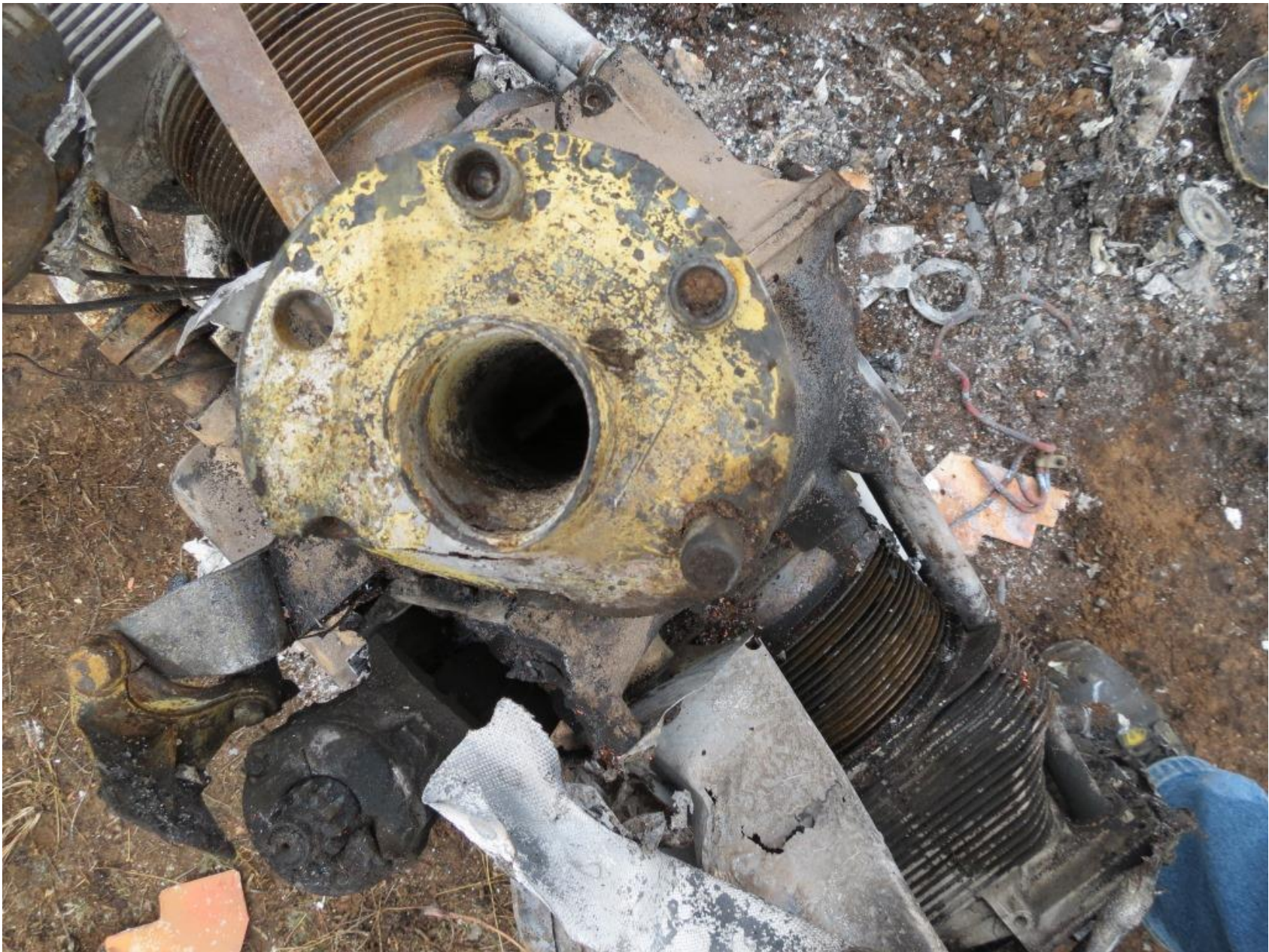
Photo 9 – View of propeller flange and cylinders
