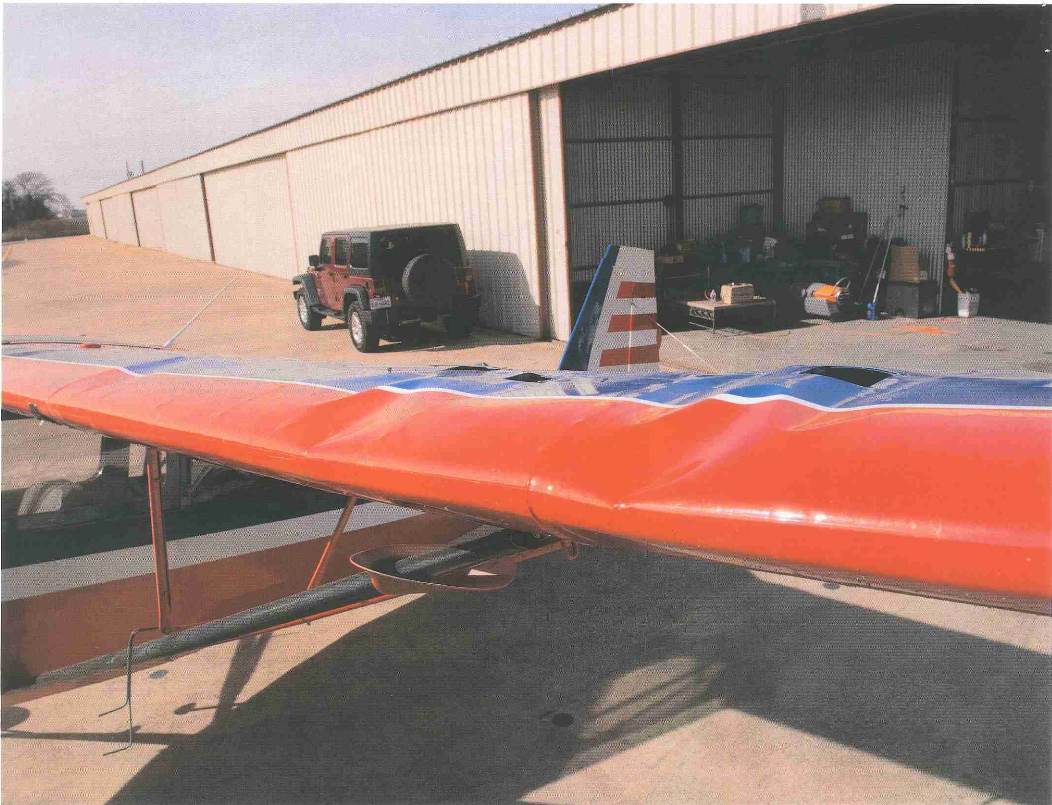
Photo 1 – Wing Damage (Photo Courtesy of FAA)
