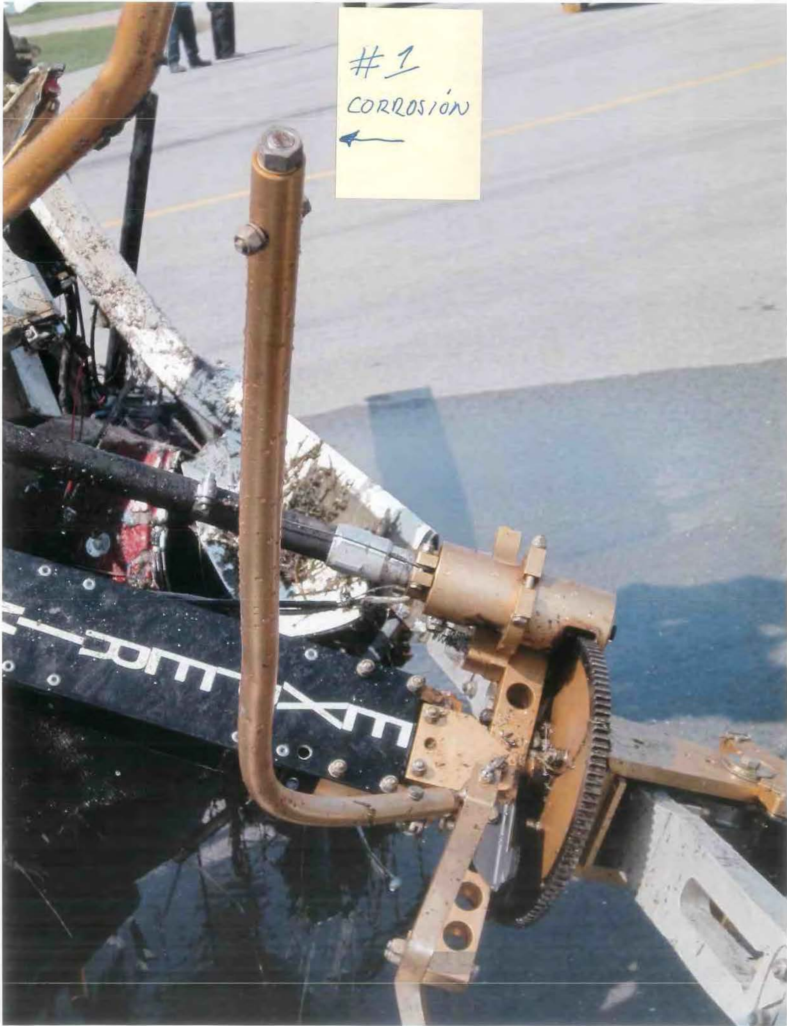
Photo 3 - Corroded Flight Control Rod Bearing
