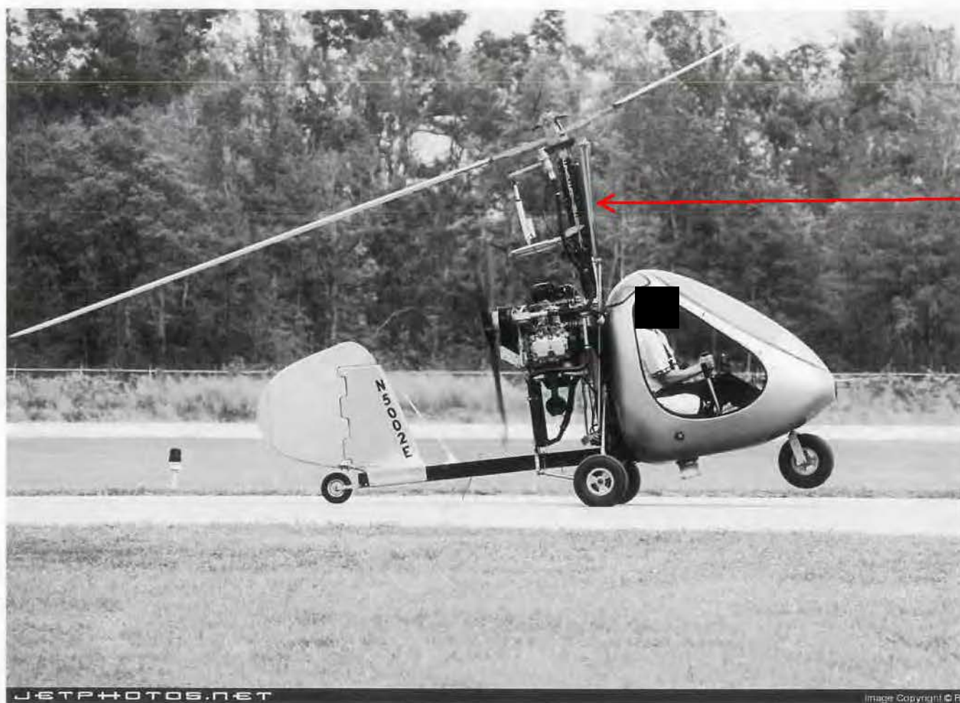
N5002E before the accident, showing the flight control that failed
