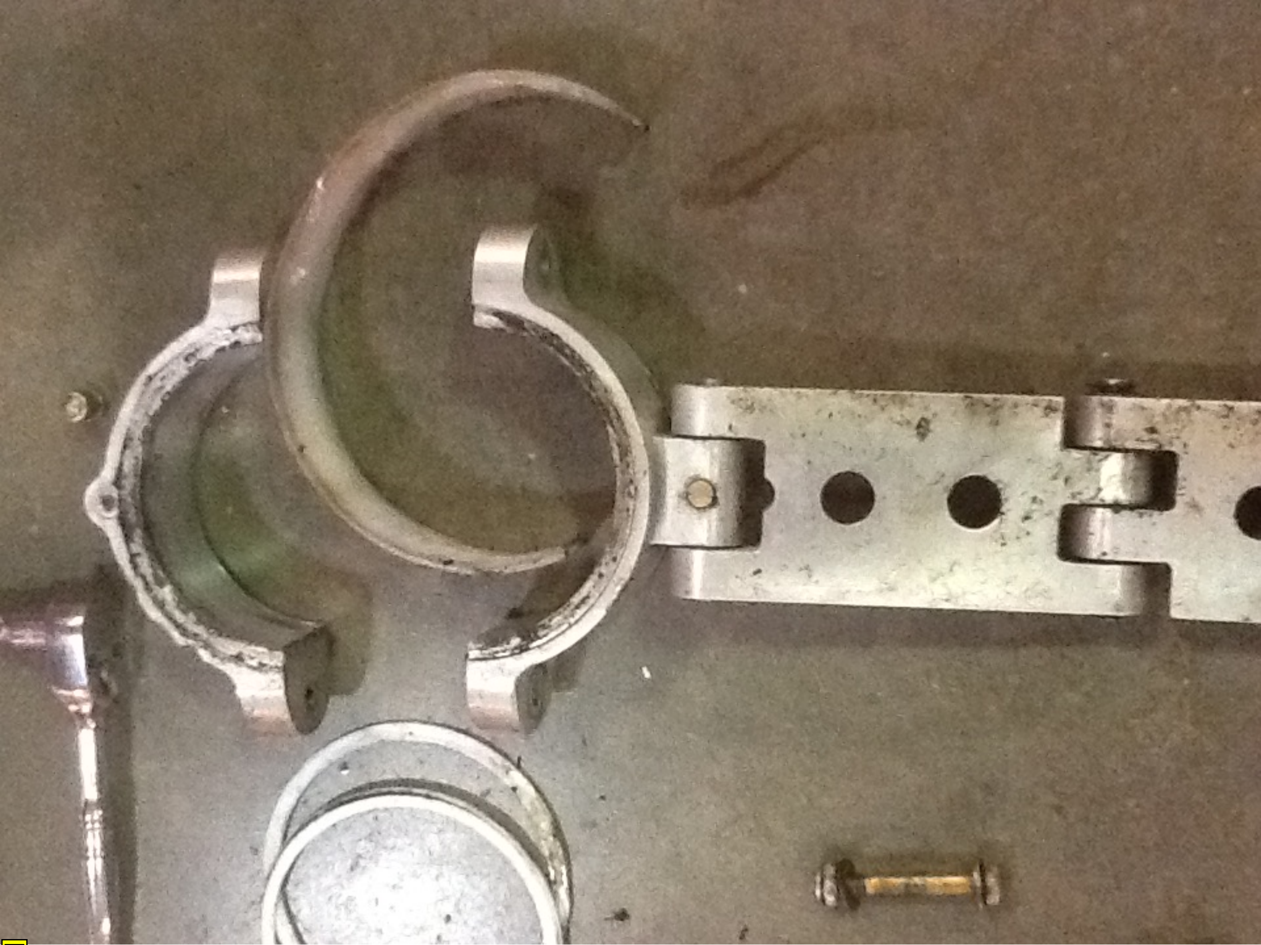
Photo 9 - Disassembled Shimmy Damper
