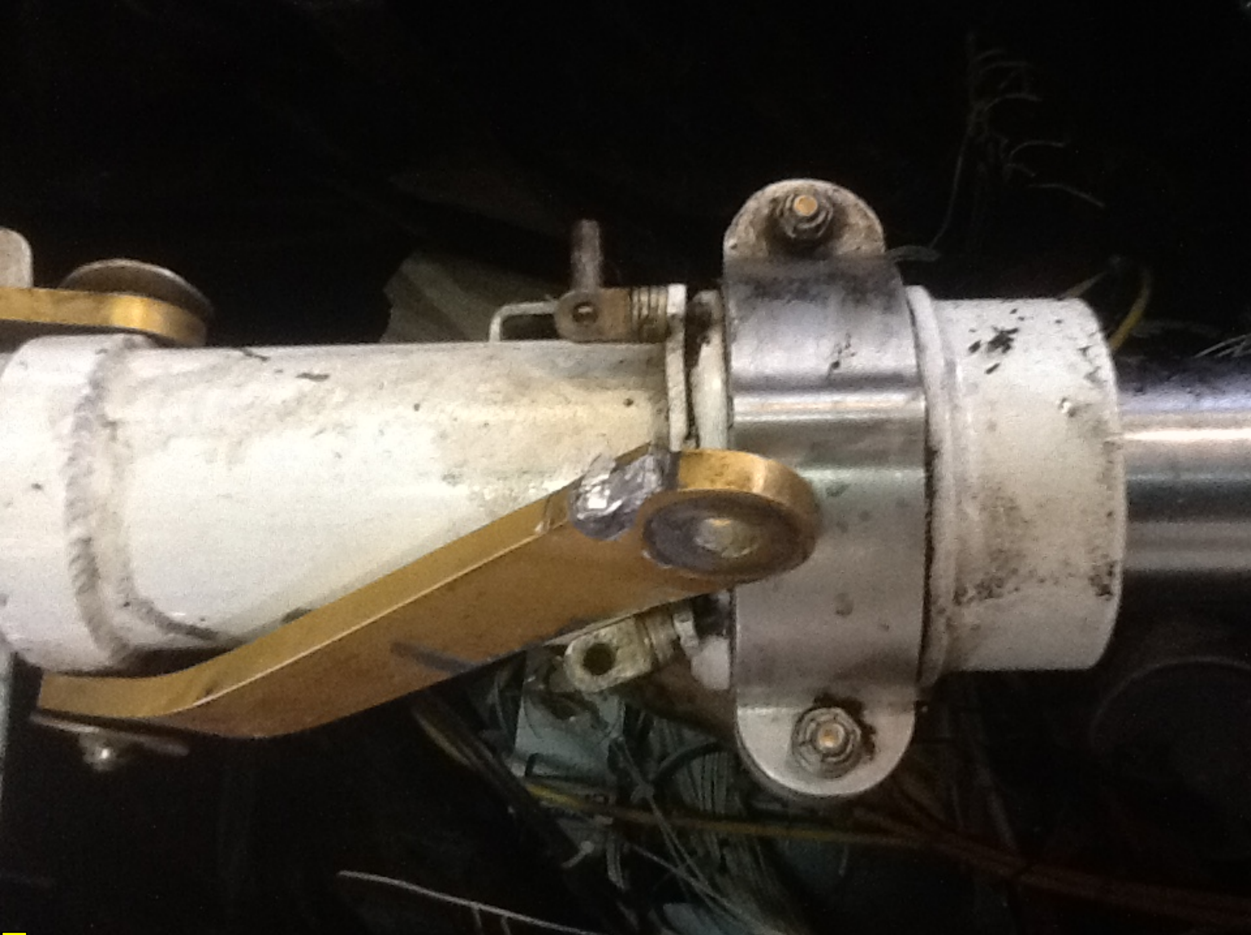
Photo 7 - Drag Link Next to Stop Pin
