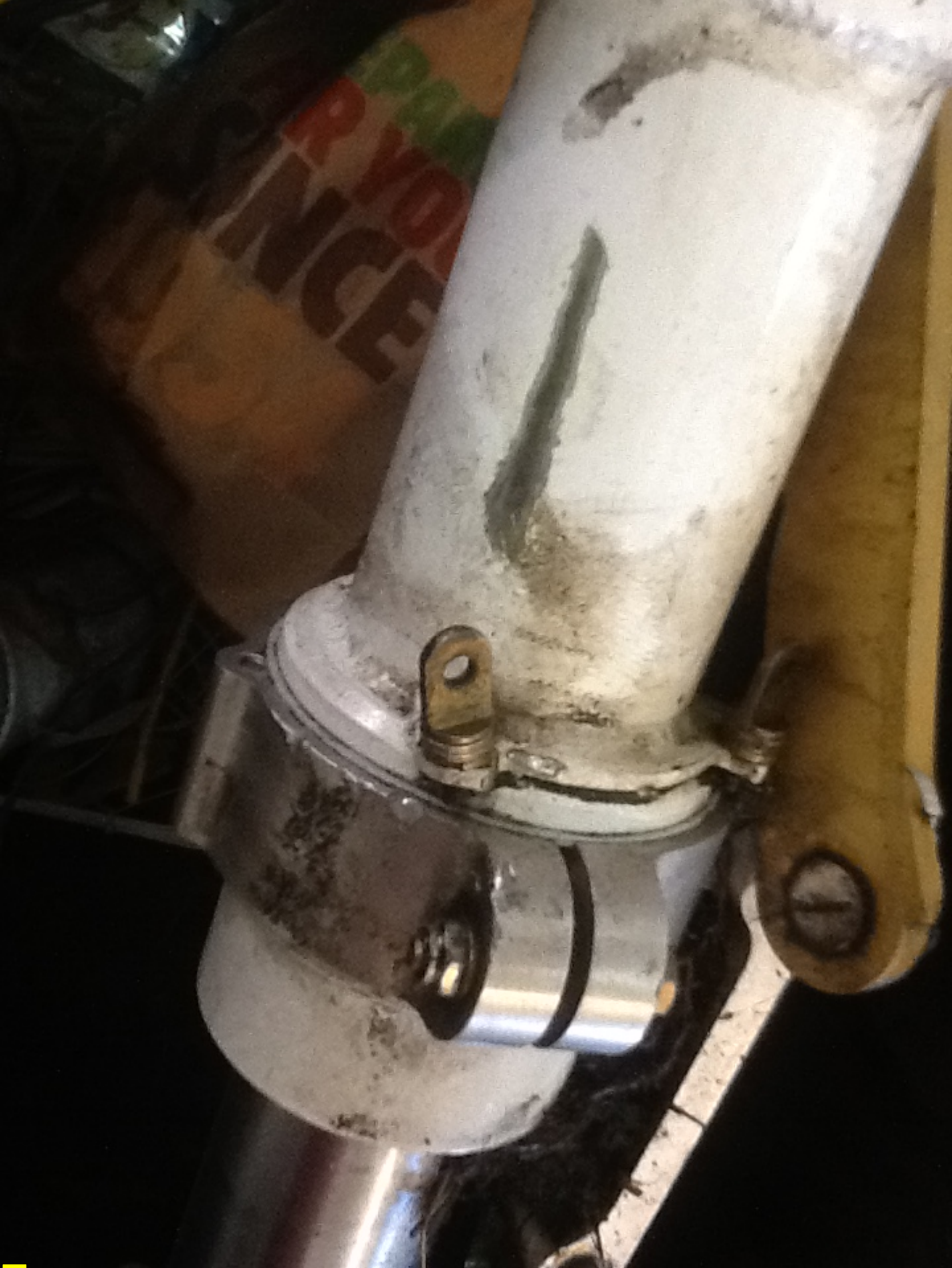
Photo 6 - Bent Travel Stop
