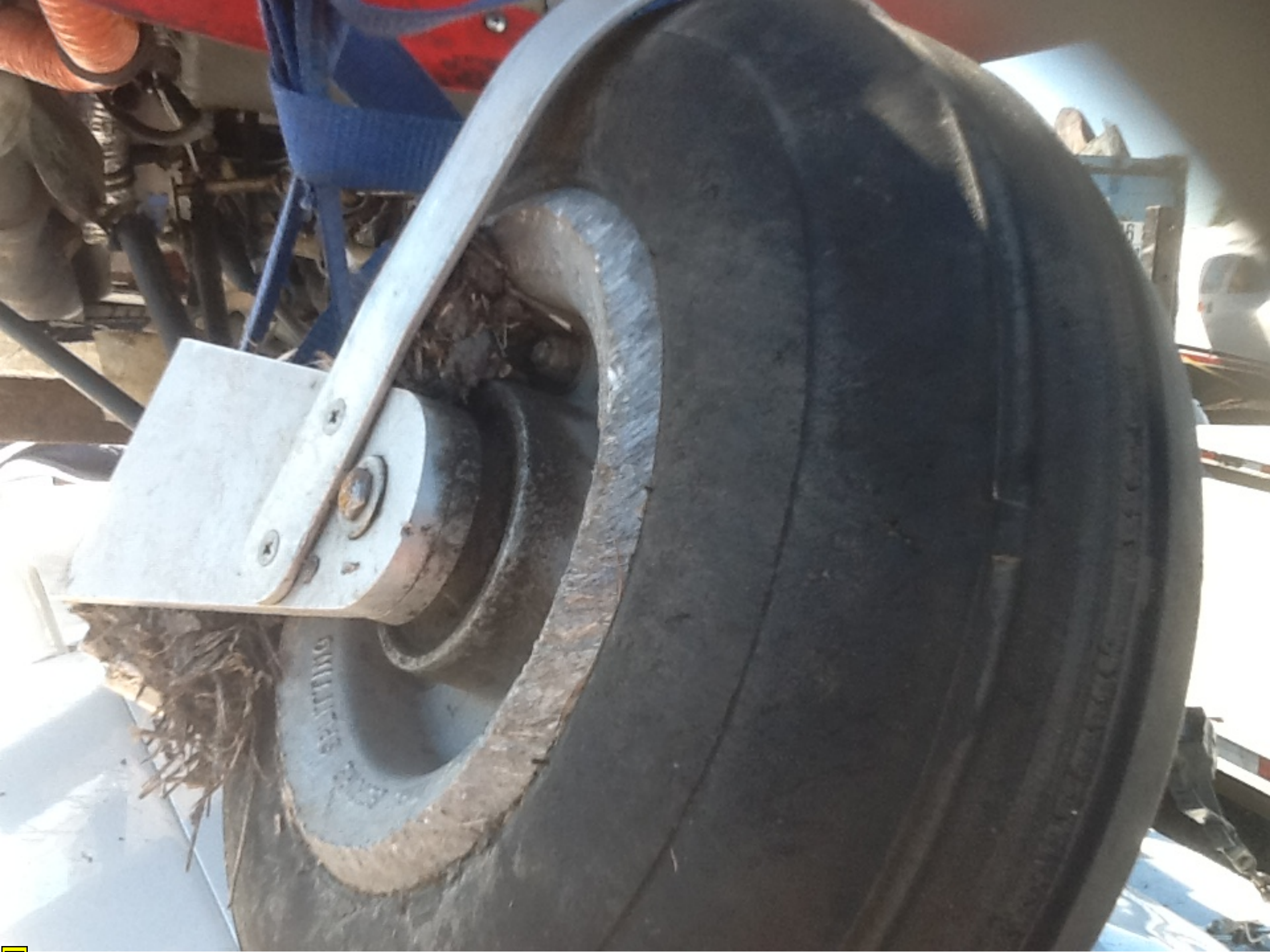
Photo 5 - Scuffed Tire and Wheel Damage
