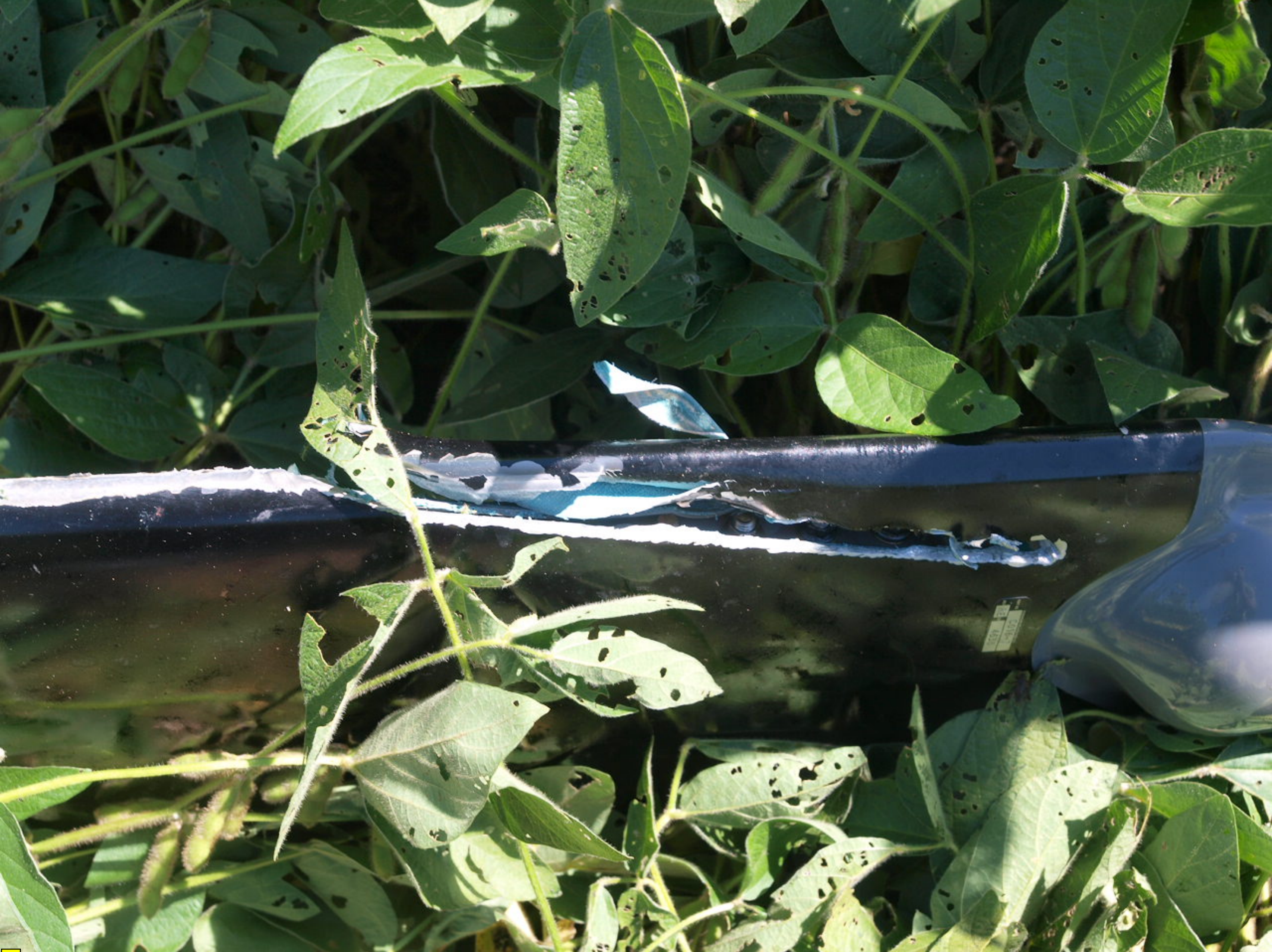
Photo 4 – Main Rotor Blade Wire Strike (FAA Photo)
