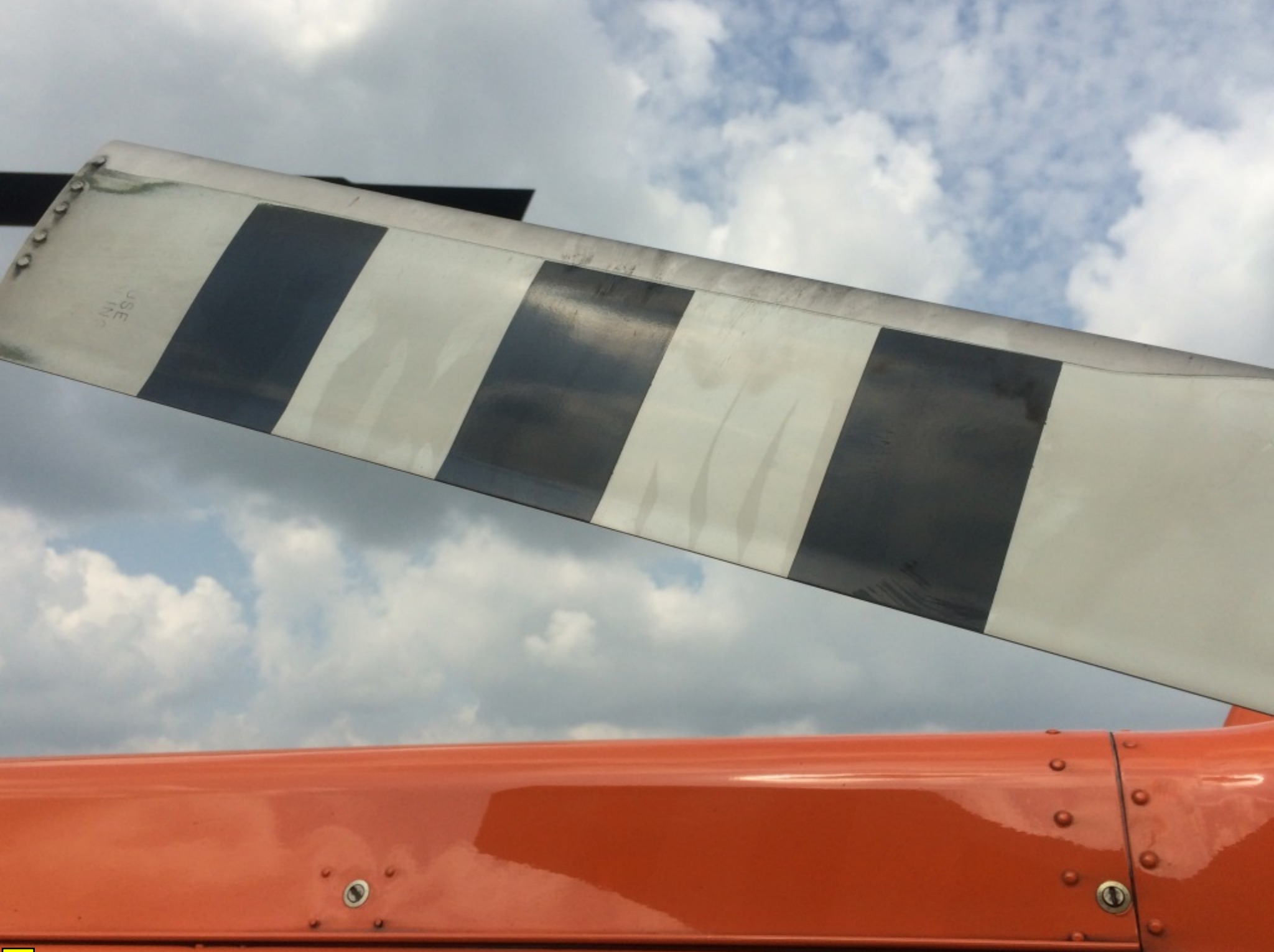
Photo 2 – View of tail rotor blade damage
