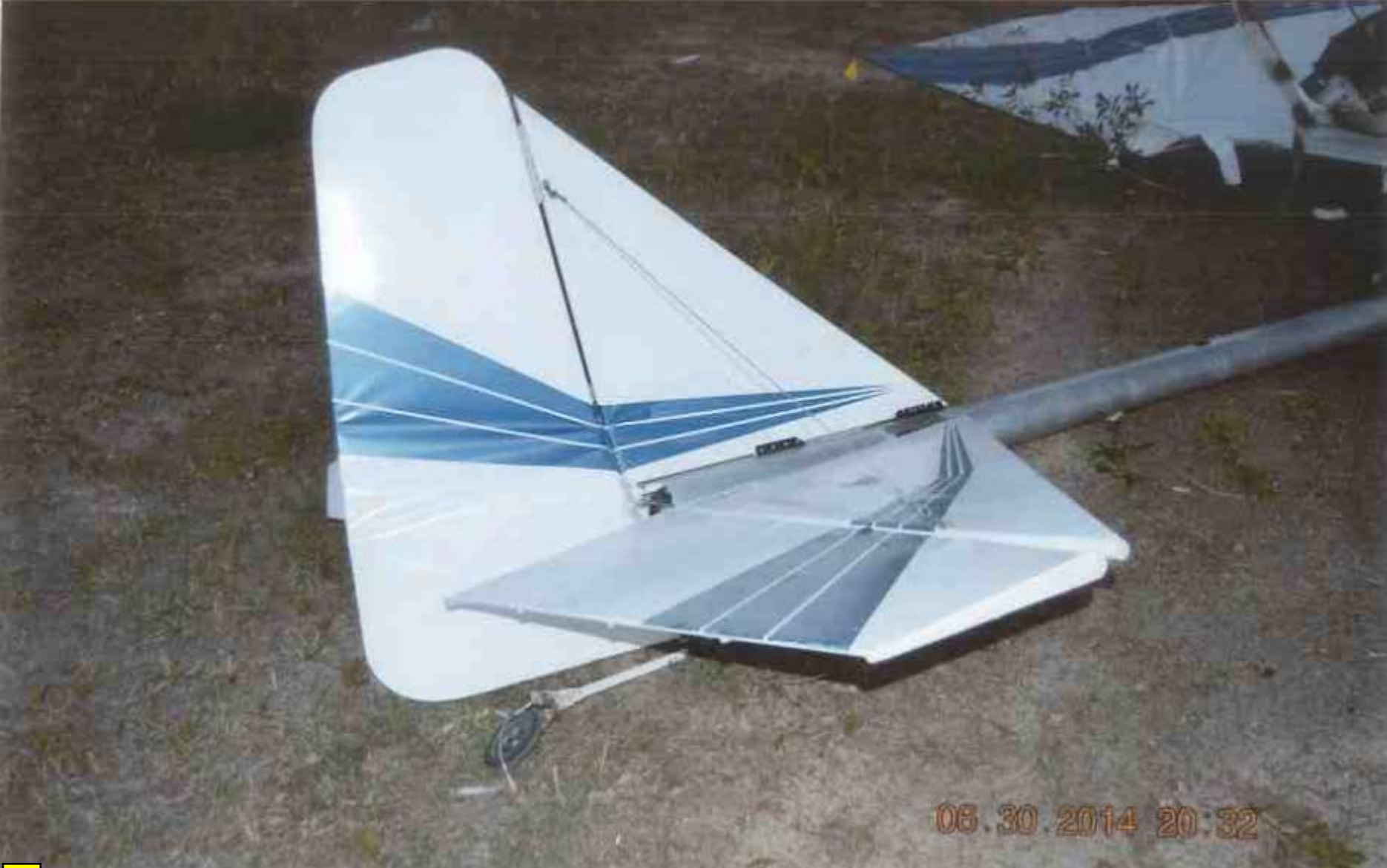
Photo 5 - Empennage (Photo Courtesy of Catahoula Parish)
