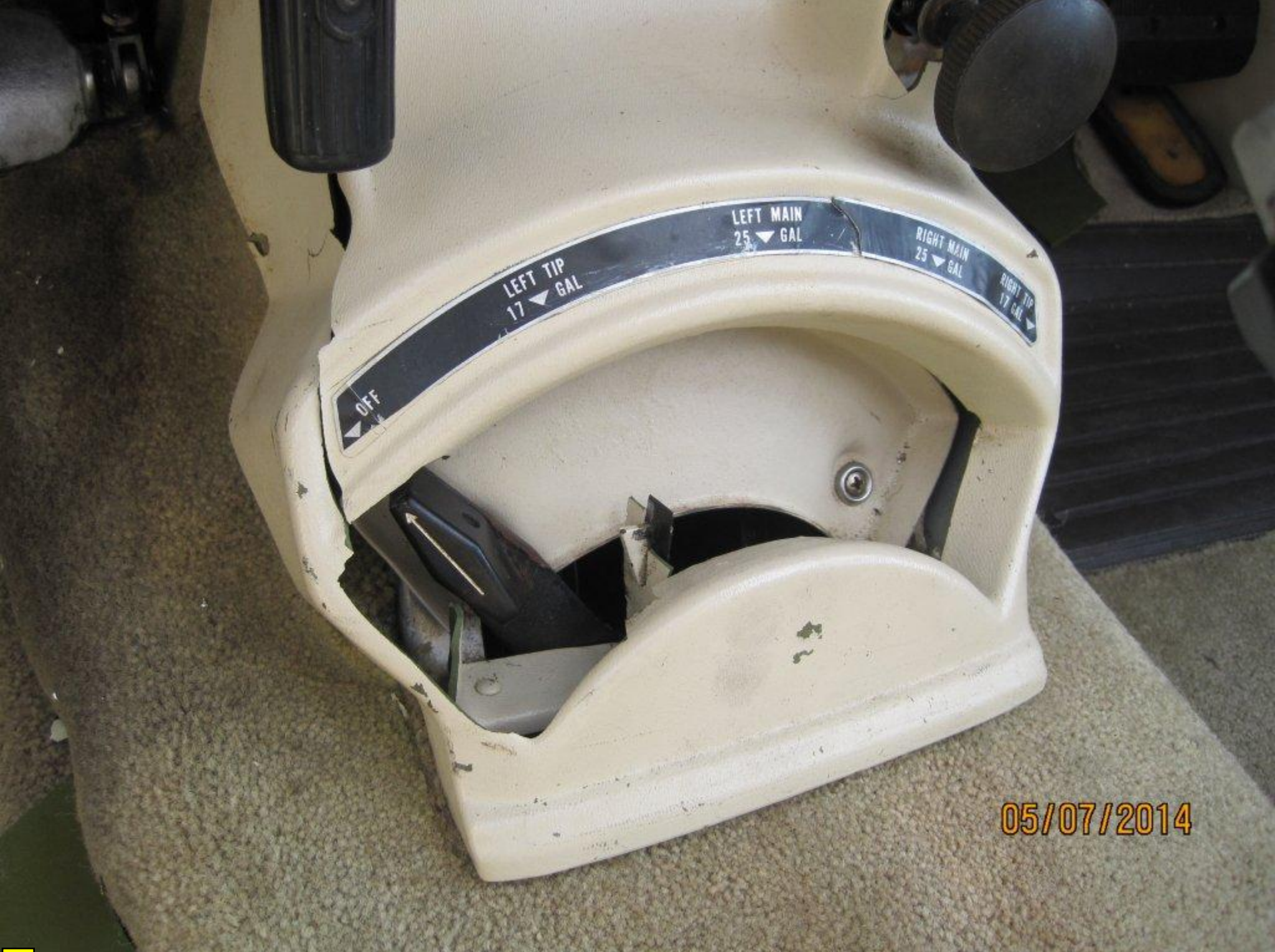
Photo 2 – Fuel Selector (Photo Courtesy of FAA)
