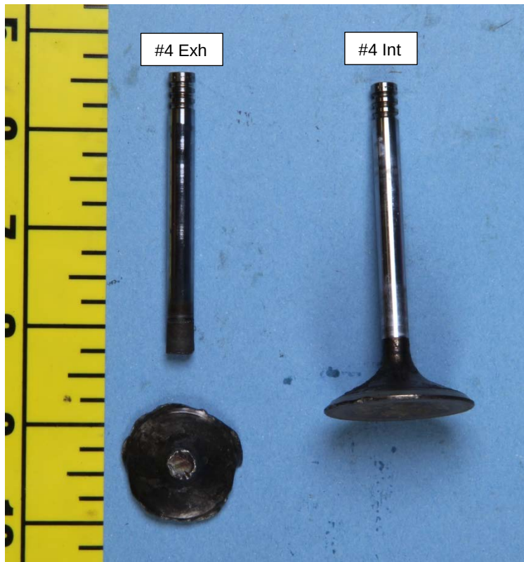
Figure 3. At left, the intake and fractured exhaust valves. A closer side view of the fractured area of the exhaust valve is shown below.
