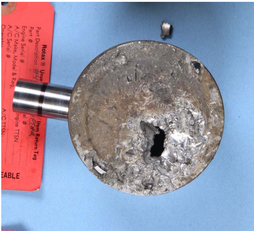
Figure 2. Views showing the impact damage to the cylinder crown and piston top.
