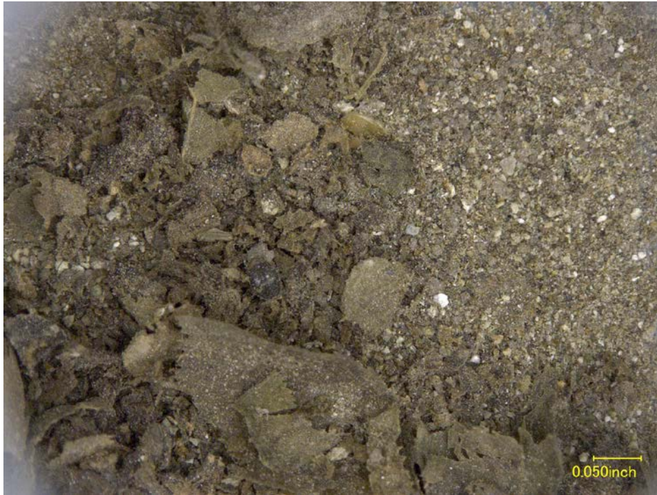
Figure 19. Photograph of material removed from cabin heater drain line.
