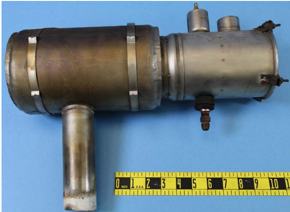
Figure 13. Photograph of cabin heater with outer cover removed.
