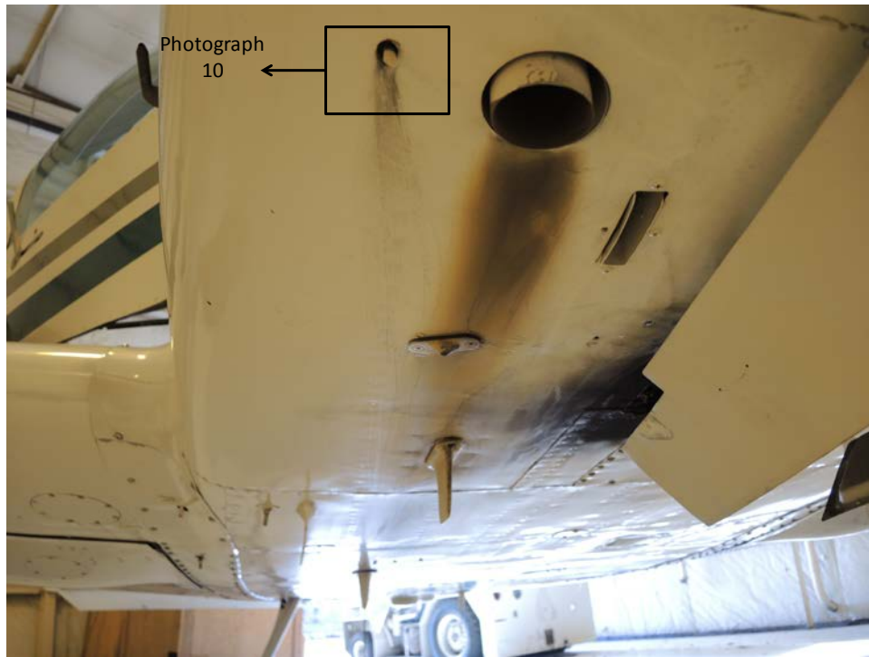
Figure 5. Close-up photograph of cabin heater exhaust and drain.
