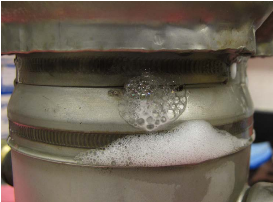
Figure 16. Photograph of leaks in combustion chamber-heat muff weld. One leak was made visible by the bubbling leak detector liquid.
