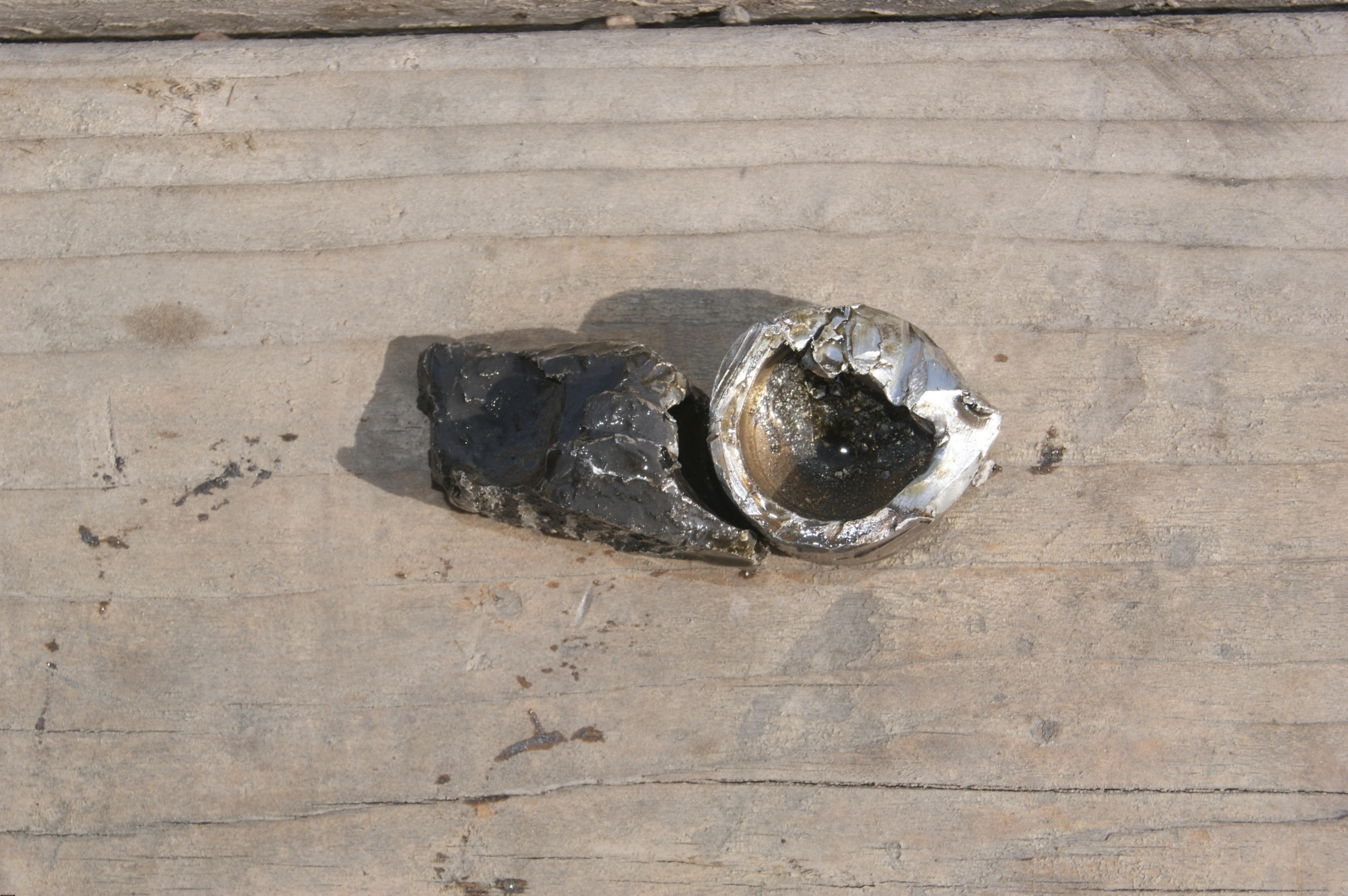
Photo 10 - Number 5 connecting rod cap (bottom view) and a portion of the connecting rod where it attaches to the piston pin
