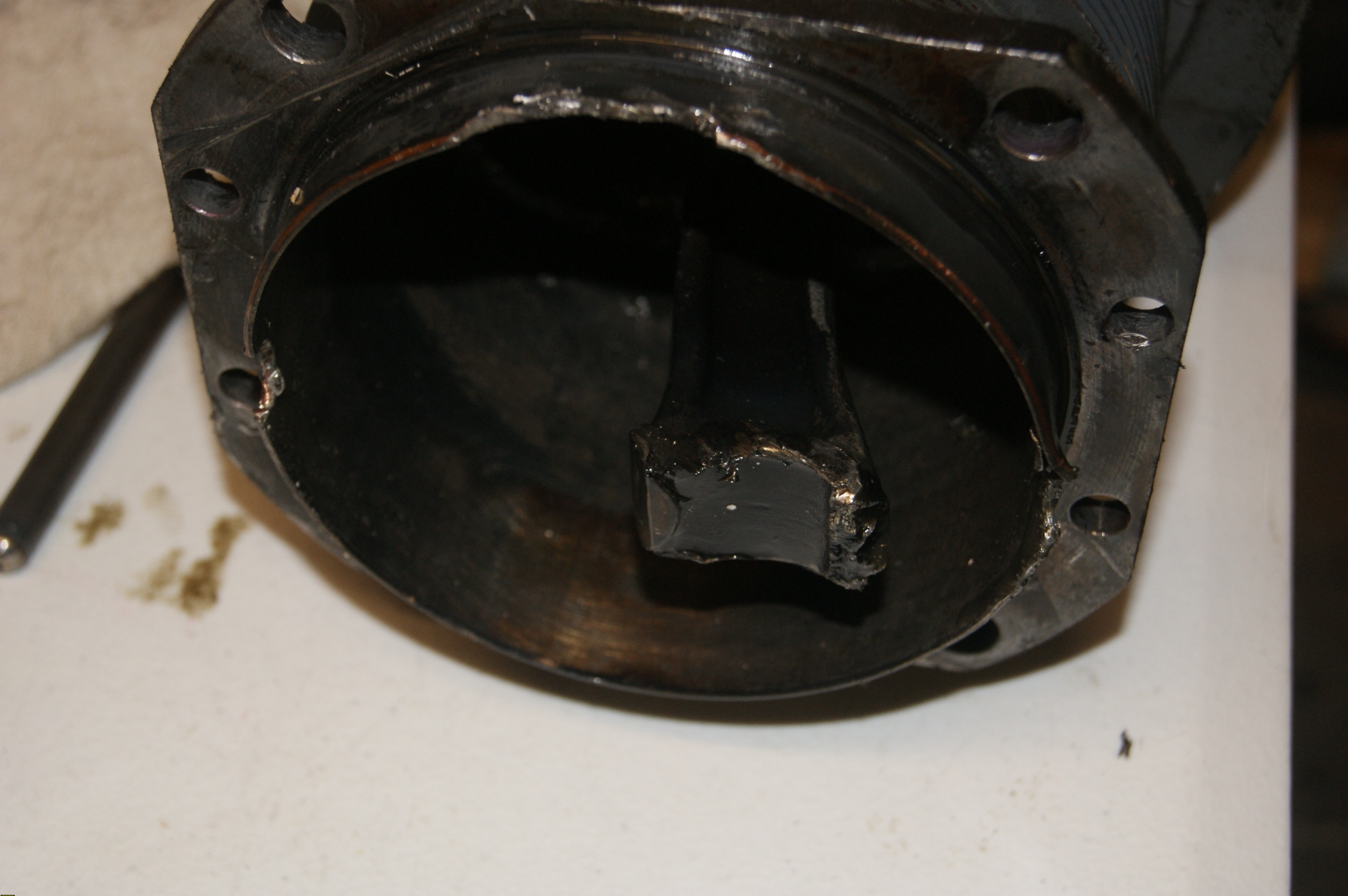
Photo 6 - Number 5 cylinder, seized piston, and fractured connecting rod cap
