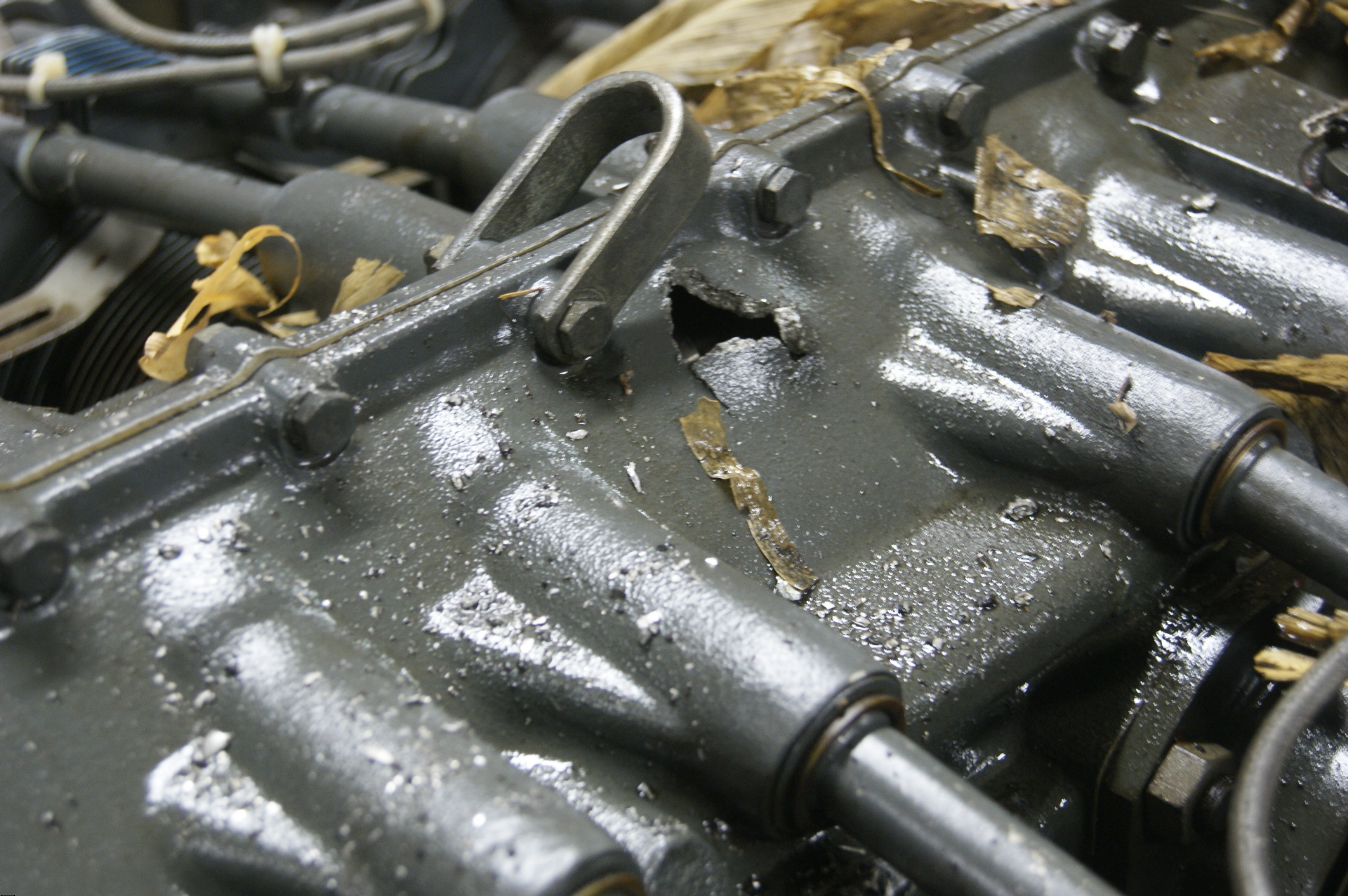
Photo 4 - Hole in top left of crankcase between numbers 2 and 4 cylinders. Note metal flakes
