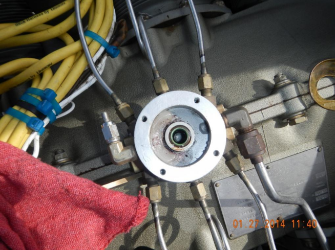
Photo 3. Ice in right fuel manifold valve (Photo Courtesy of Continental Motors)
