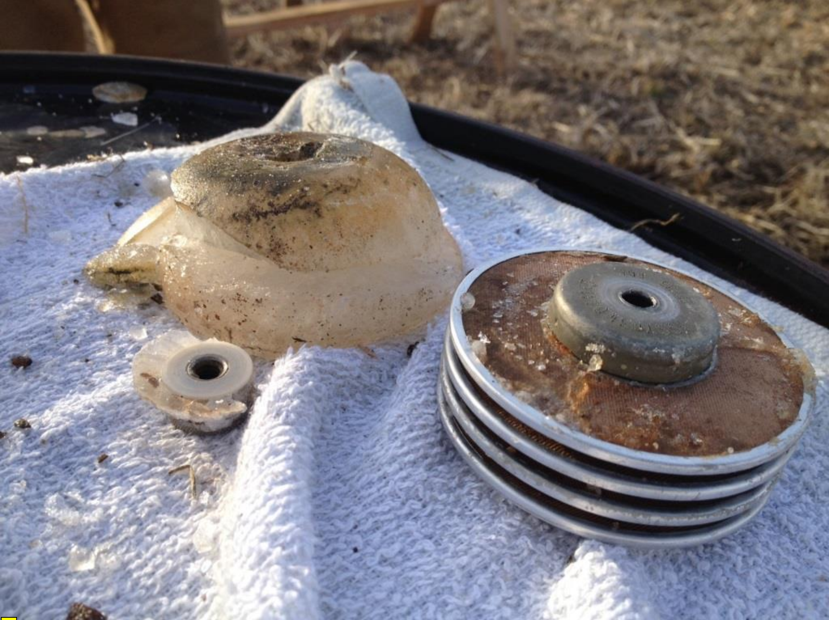
Photo 1. Ice from right fuel strainer bowl (Photo Courtesy of Continental Motors)
