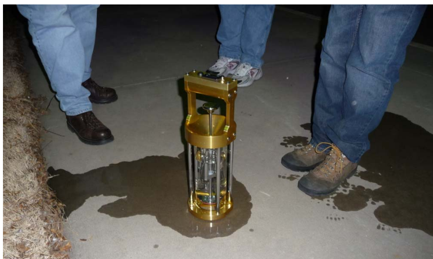
Figure 3: Water outflow meter (Hydrotimer) demonstration test on RIAC sidewalk pavement leading to the airport terminal.
