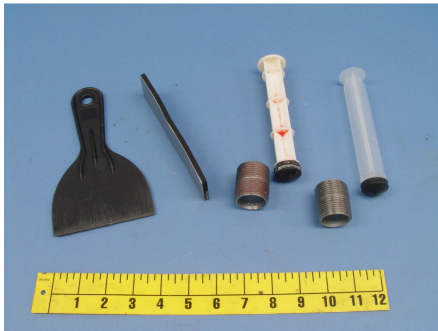
Figure 2: Grease test equipment including, from left to right, 4-inch-wide plastic scraper, NASA 2-inch-wide rubber squeegee, cylinder and rubber-tipped plunger to measure and apply known Boeing grease volume to test station, cylinder and rubber-tipped plunger to measure and apply known NASA grease volume to test station.
