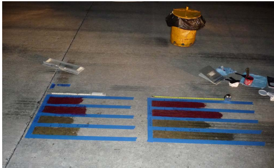
Figure 5: Grease sample test results at the station 6,000 feet from the runway 21 threshold, 17' left of centerline for Operator 2 (NASA technical consultant, left) and Operator 1 (NTSB, right).
