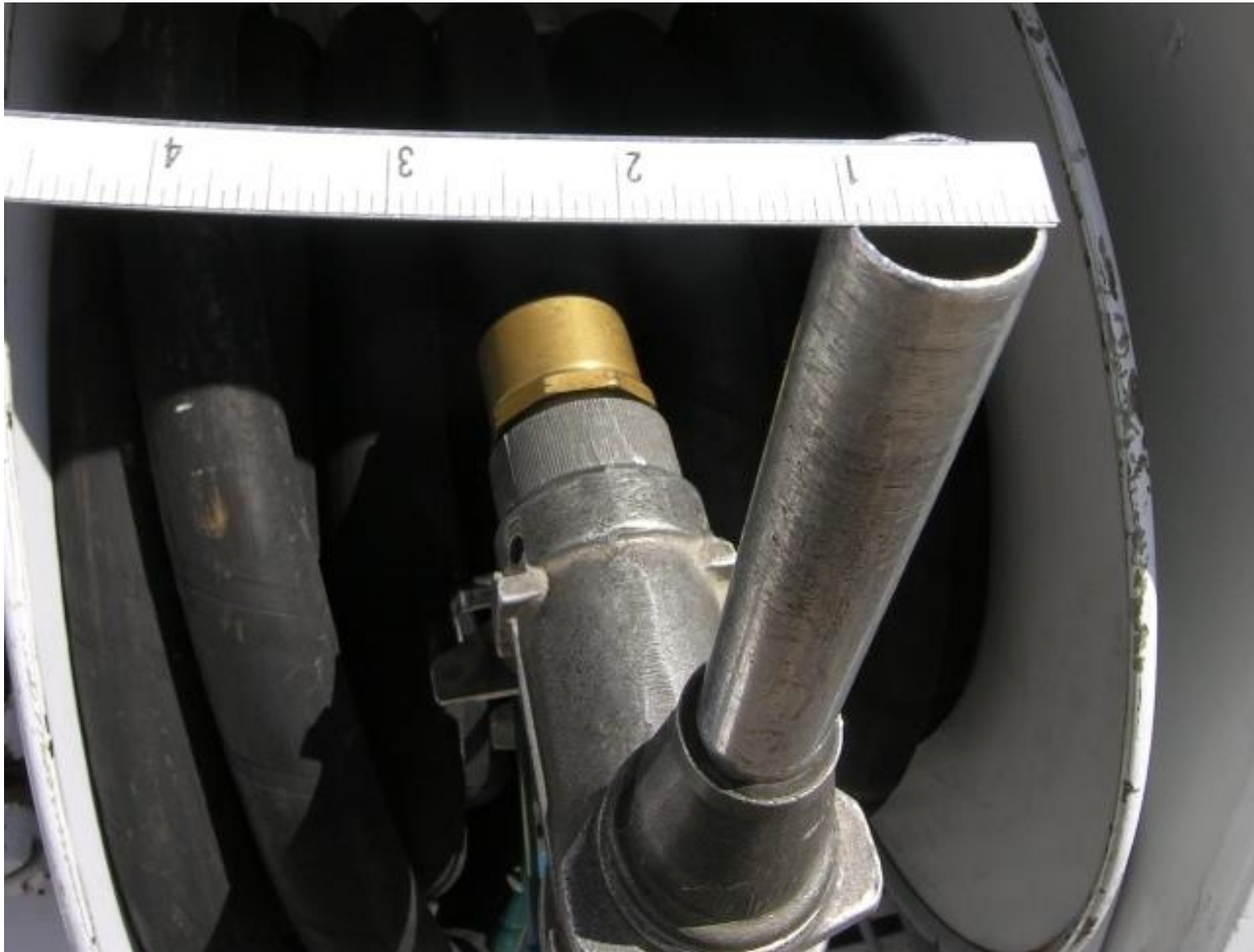
Photo 8 - LRU airport – 1 inch diameter Avgas fuel nozzle (NTSB Photo)
