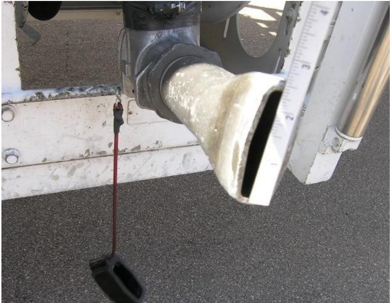
Photo 10 - LRU airport – 2 ½ inch wide “Duckbill” Jet fuel nozzle (NTSB Photo)
