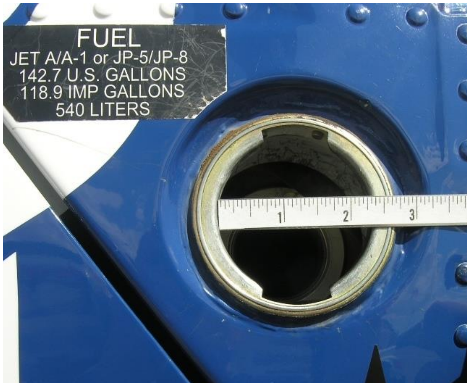
Photo 11 – LRU airport – 2 ¼ inch diameter fuel port on an AS-350 helicopter (NTSB Photo)
