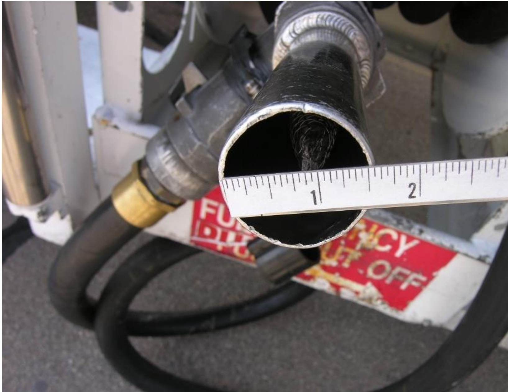
Photo 9 - LRU airport – 1 5/8 inch diameter Jet fuel nozzle (NTSB Photo)
