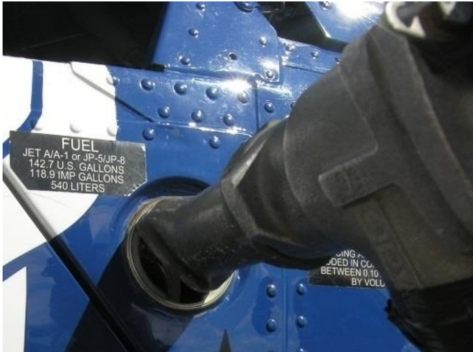
Photo 12 - LRU airport – “Duckbill” fuel nozzle shown next to the 2 ¼ inch diameter fuel port on an AS-350 helicopter (NTSB Photo)
