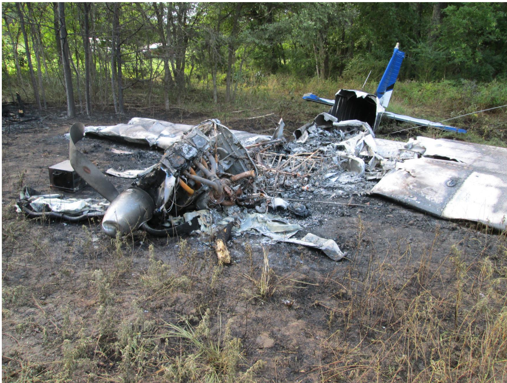
Photo 1 – View of wreckage from left front. The wreckage is in a small clearing; the engine, wings, and tail section are easily identified. The cabin area has been mostly consumed by fire.
