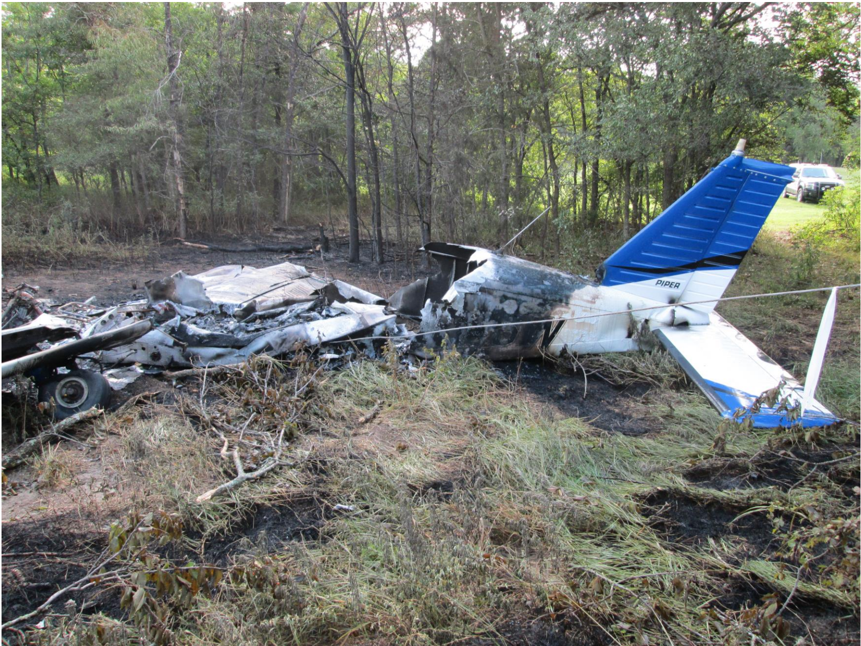
Photo 2 - A left side view of the wreckage. Much of the cabin has been consumed by fire. A power cable can be seen, in the photograph.
