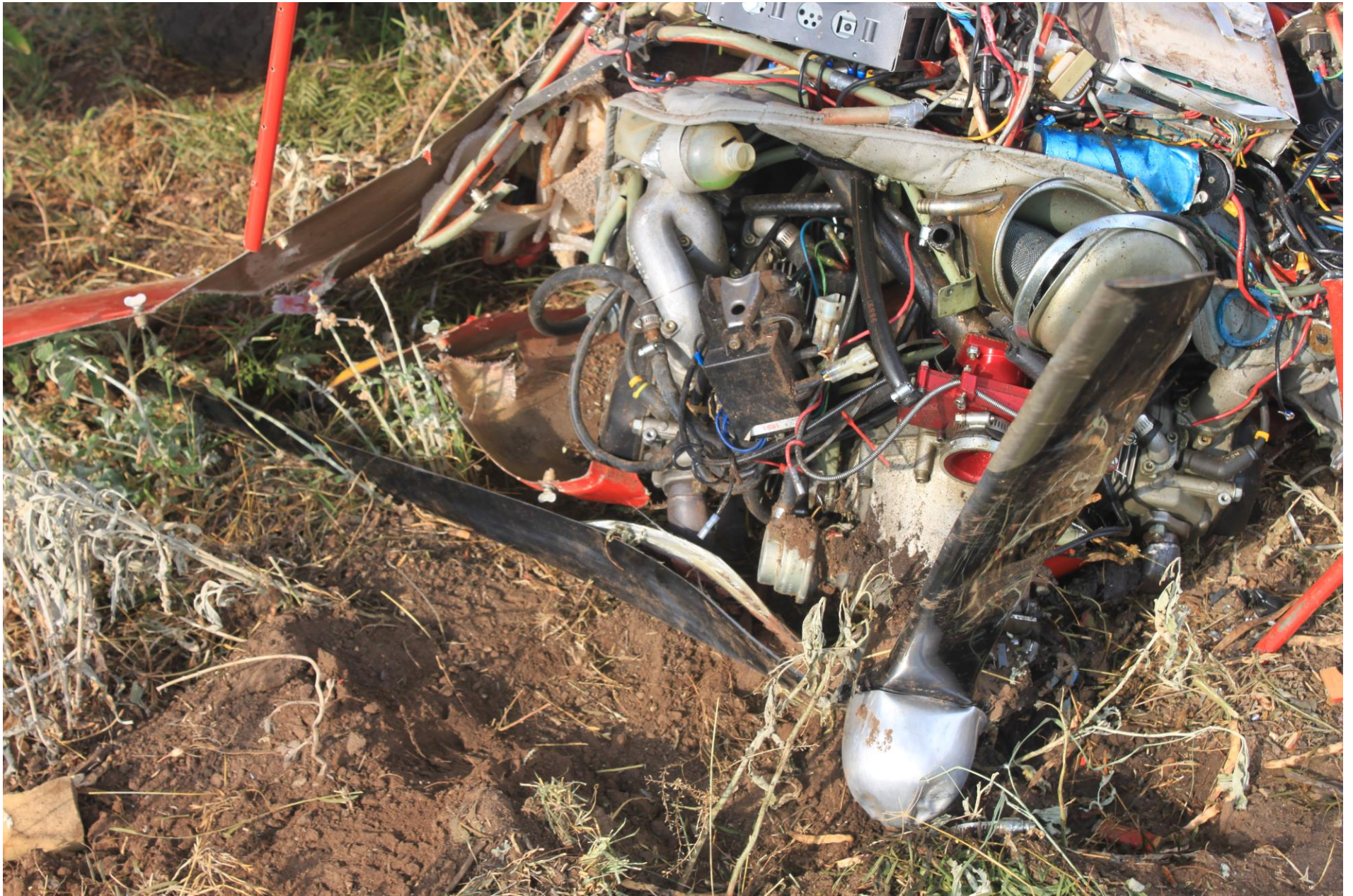
Photo 7 – Propeller and Ground Witness Mark
