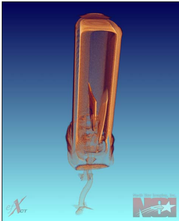
KC 192: Y101 crystal CT scan images show that the piezoelectric disk is broken – consistent with impact forces (conducted in Phoenix, Arizona)
