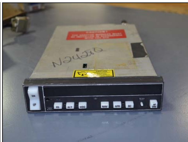
KC 192 front and top views: no damage detected
