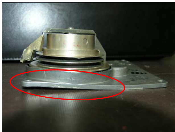
KM 275 Servo Mount: side view, base plate distorted as shown
