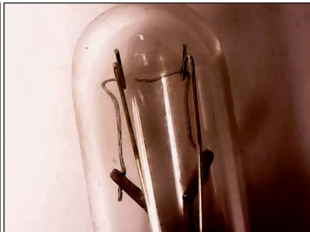
AP lamp: filament broken, no stretching (no spaghetti appearance)
