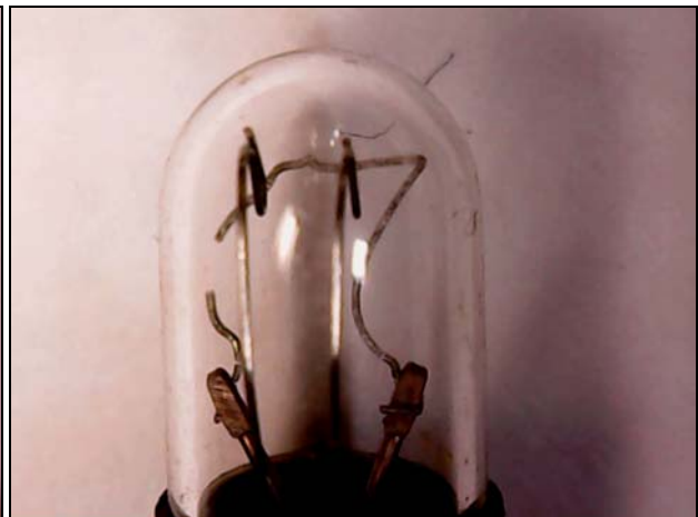
HDG lamp: filament broken, no stretching (no spaghetti appearance)
