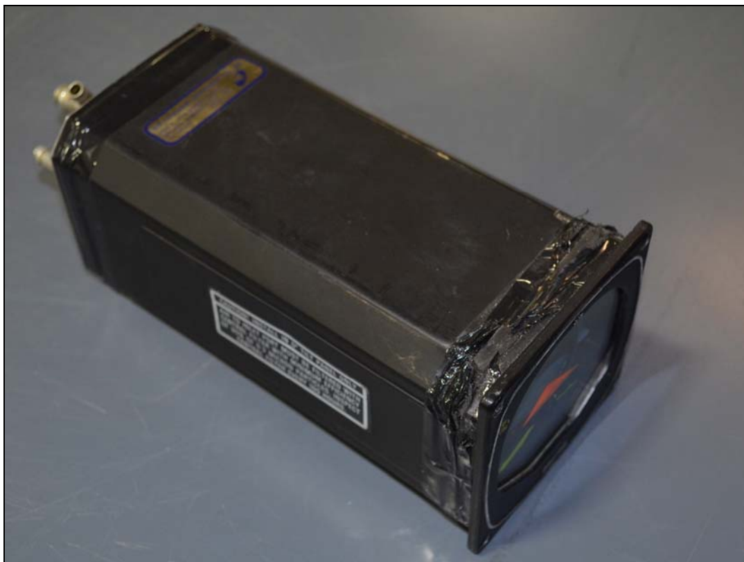
KI 256 – no apparent physical damage observed in this view
