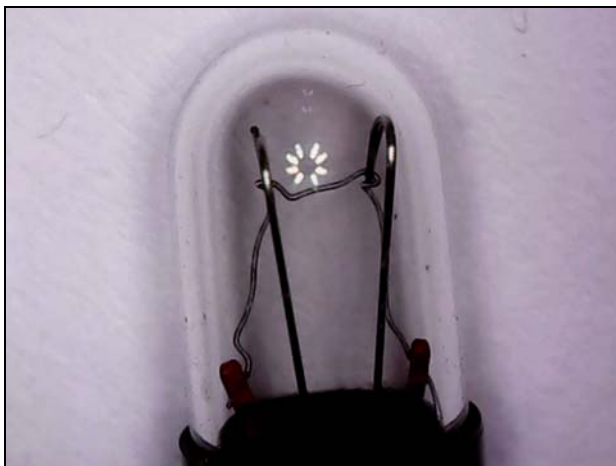
GS lamp: filament not broken, no stretching (no spaghetti appearance)
