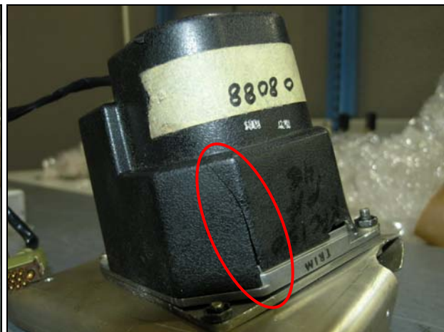
KS 272A Trim Servo: cover cracked
