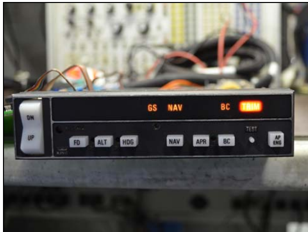
KC 192 self test: YD, FD, ALT, HDG, APR and AP lamps out
