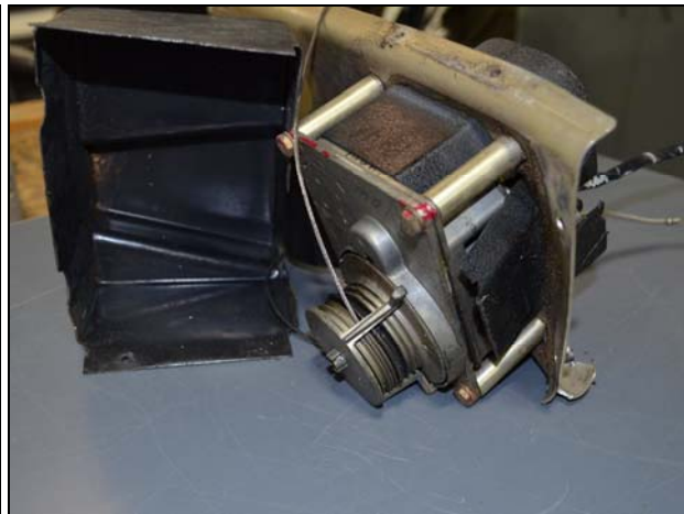
KS 271A Yaw Servo with associated KM 275 mount, cover, and bracket
