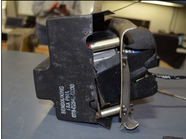
KS 271A Primary Servo (Yaw): cover damaged and partially broken away exposing internal parts/structure
