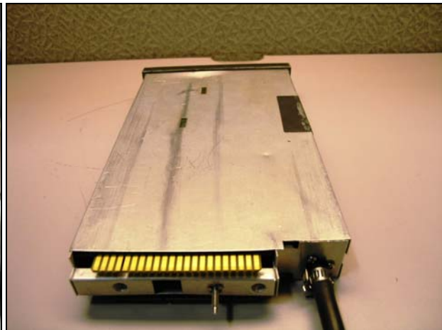
KC 192 rear and bottom views – no damage detected
