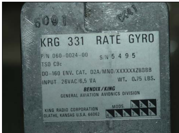
KRG 331 Rate Gyro (Yaw) dataplate: P/N 060-0024-00, S/N 5495
