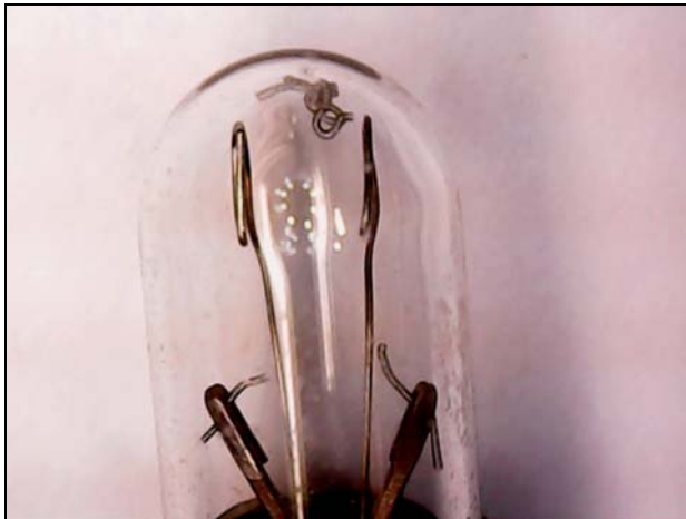
YD lamp: filament broken, no stretching (no spaghetti appearance)
