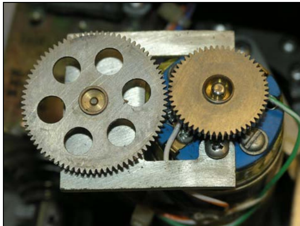
KS 271A Pitch Servo: tach motor shaft and mounting bracket bent – straightened later to allow gear engagement and testing
