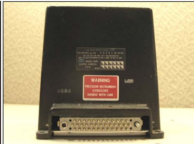
KG 102A rear view – no visible damage detected
