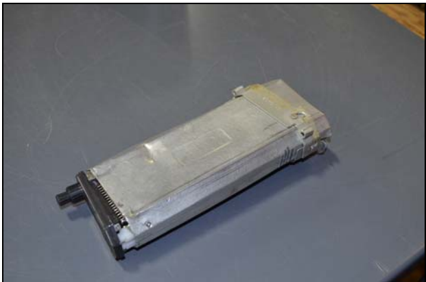
KAS 297B Altitude/VS Selector: cover, connector, bezel, and chassis damage/deformation
