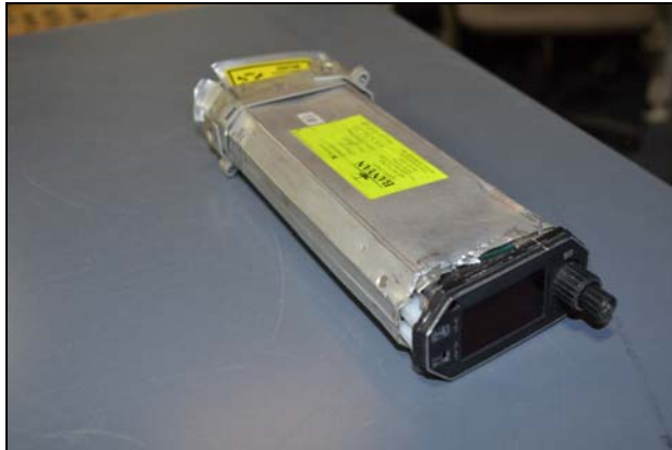
KAS 297B Altitude/VS Selector: cover, connector, bezel, and chassis damage/deformation
