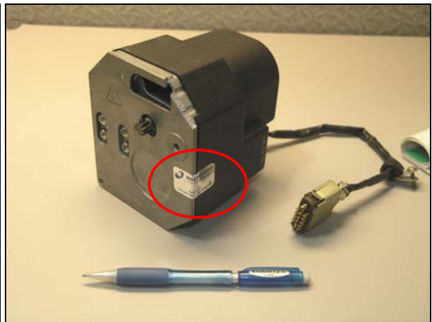
KS 271A Roll Servo: Midcontinent Instruments integrity seal intact
