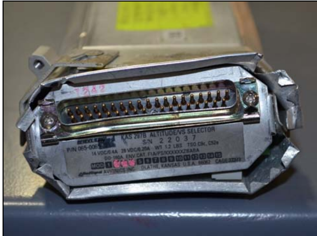
KAS 297B rear connector damaged
