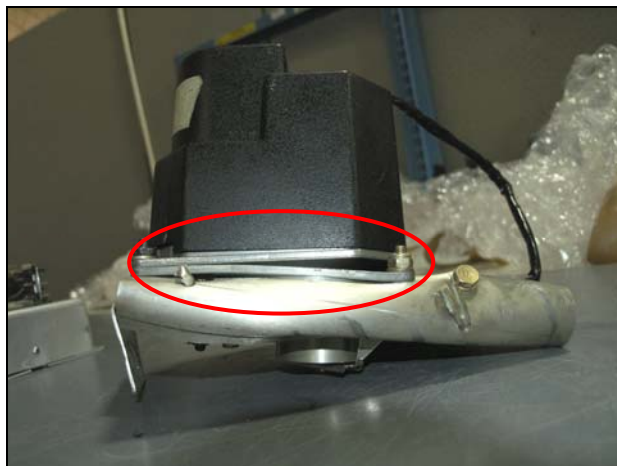
KS 272A Trim Servo and KM 275 mount: mount twisted
