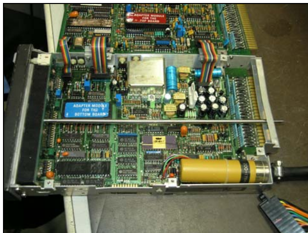
KC 192 top board – no damage detected
