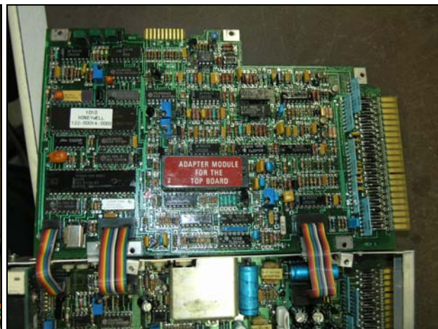
KC 192 bottom board – no damage detected
