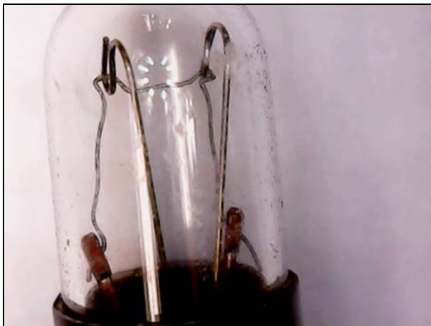
TRIM lamp: filament not broken, no stretching (no spaghetti appearance)
