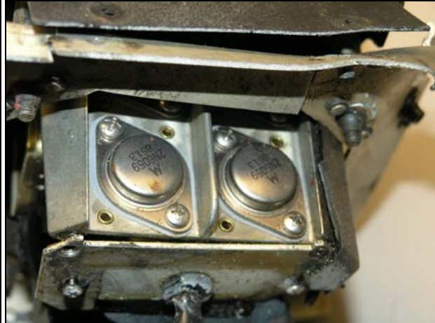
KS 271A Primary Servo (Yaw): cover damaged and partially broken away exposing internal parts/structure
