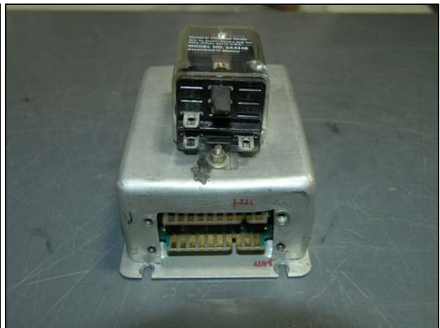
KC 296 Yaw Computer: relay attached to the cover is NOT part of the KC 296 Yaw Computer
