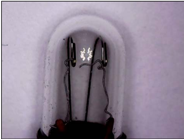
APR lamp: filament broken, no stretching (no spaghetti appearance)
