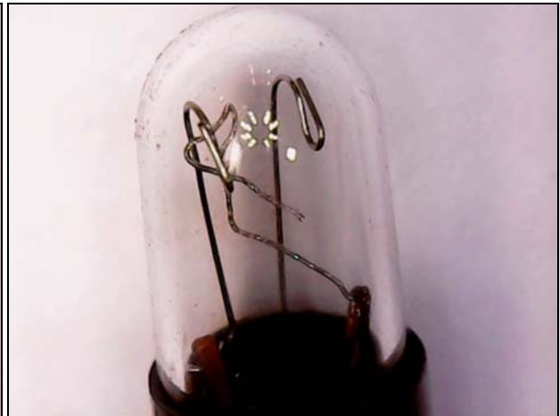
FD lamp: filament broken, no stretching (no spaghetti appearance)
