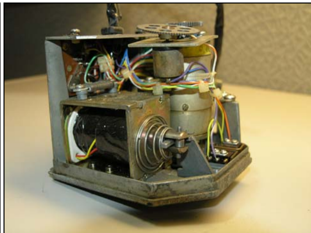
KS 271A Pitch Servo: cover missing
