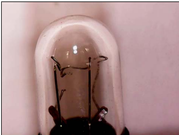
ALT lamp: filament broken, no stretching (no spaghetti appearance)
