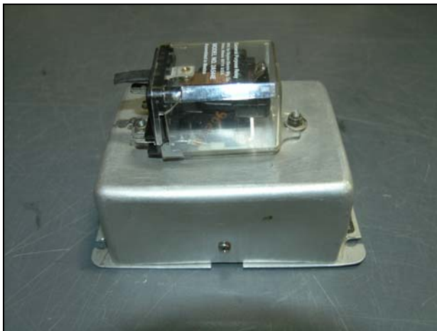
KC 296 Yaw Computer: relay attached to the cover is NOT part of the KC 296 Yaw Computer
