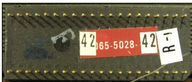
Top board adapter module: P/N 065-5028-42
