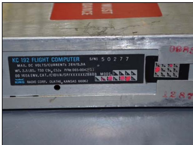
KC 192 dataplate: P/N 065-0042-03, S/N 50277, date code 0985
