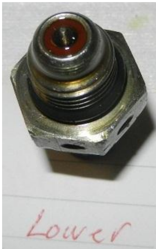
Fig 18: Lower Chip Detector
