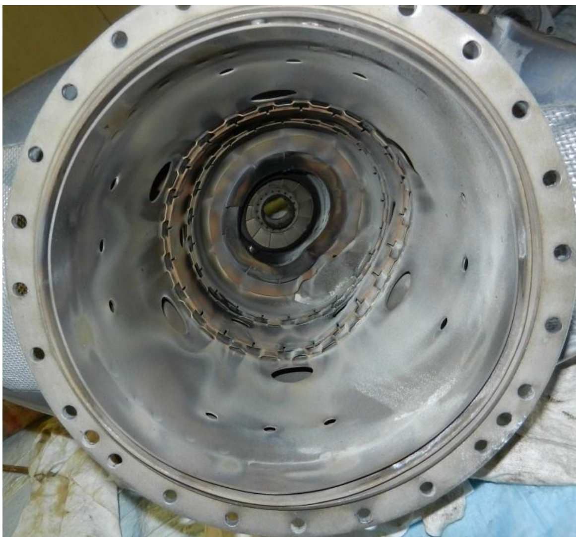
Fig 15: Impact Damage to the Combustion Liner
