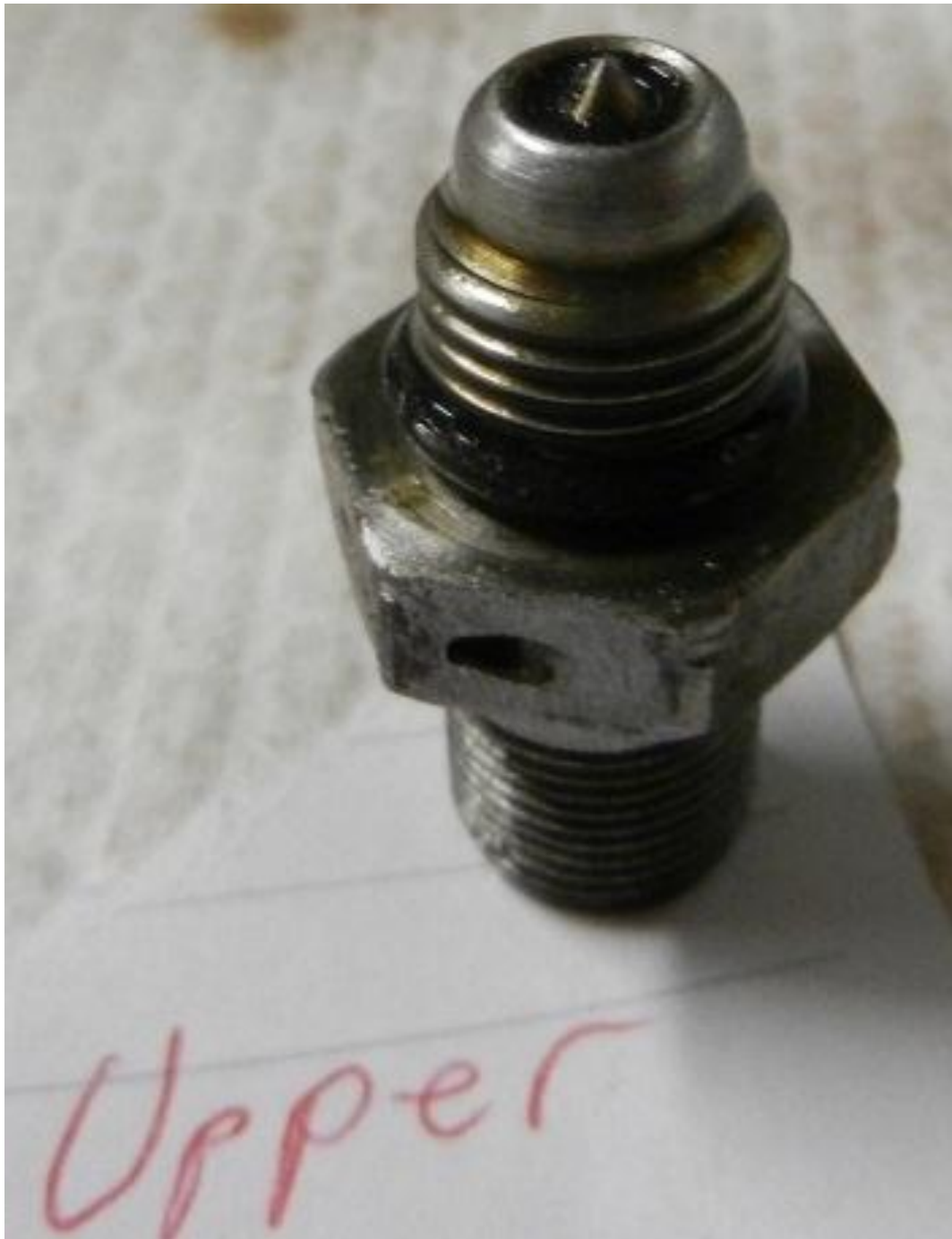
Fig 17: Upper Chip Detector
