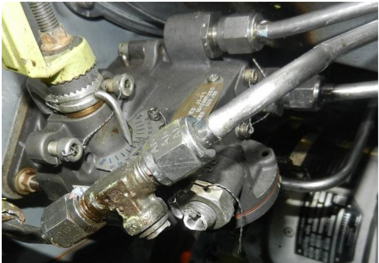
Fig 19: Power Turbine Governor
