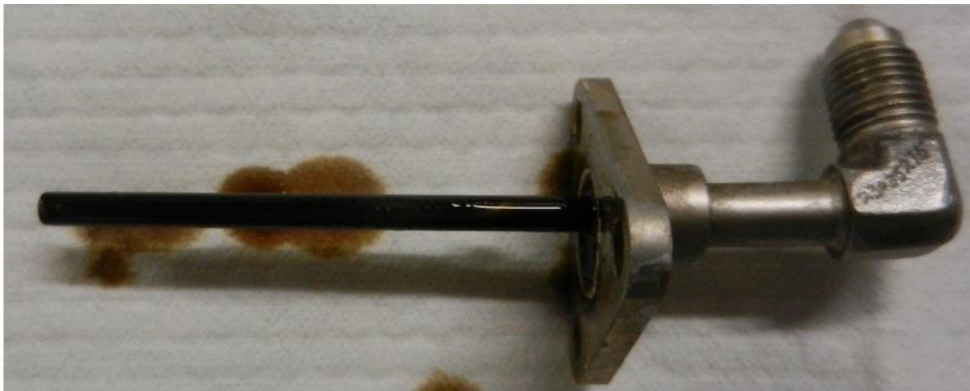
Fig 14: No. 8 Bearing Oil Delivery Tube
