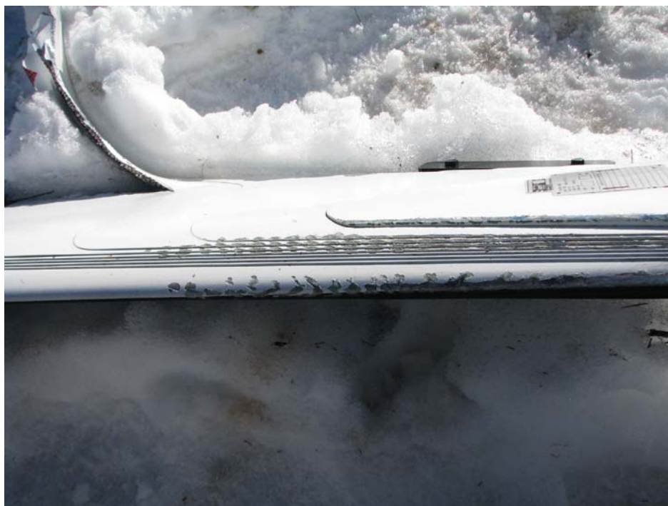
Photo 15 Scoring marks on inboard Red blade consistent with wirestrike
