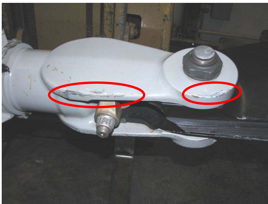
Photo 16 Red grip leading edge abrasions consistent with wire contact
