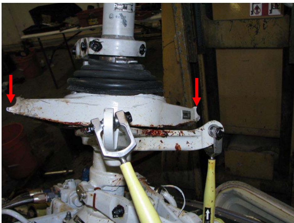
Photo 10 Both outer ring swashplate ears fractured consistent with overload forces
