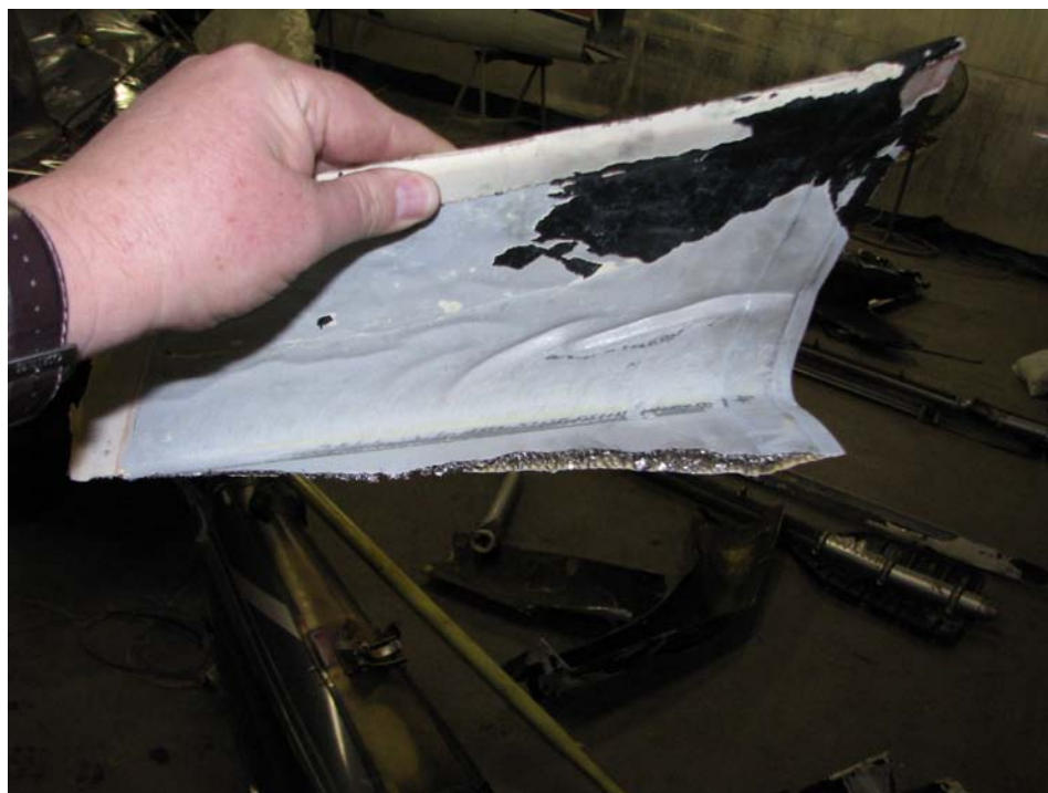
Photo 5 End plate with main rotor blade strike
