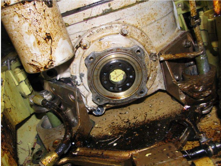
Photo 22 Input flange to main transmission
