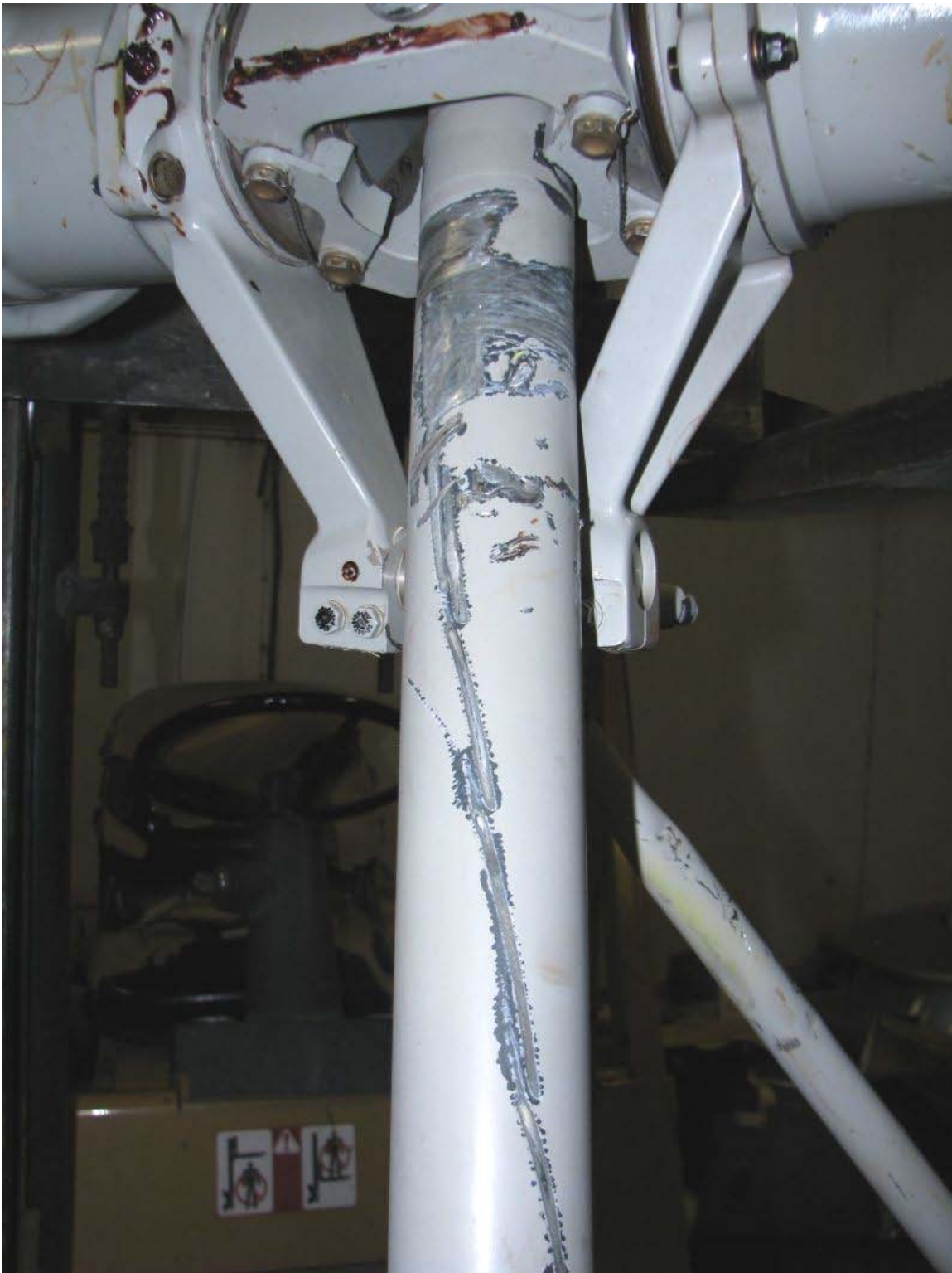
Photo 21 Wirestrike scoring marks on mast terminate at bottom of main rotor hub
