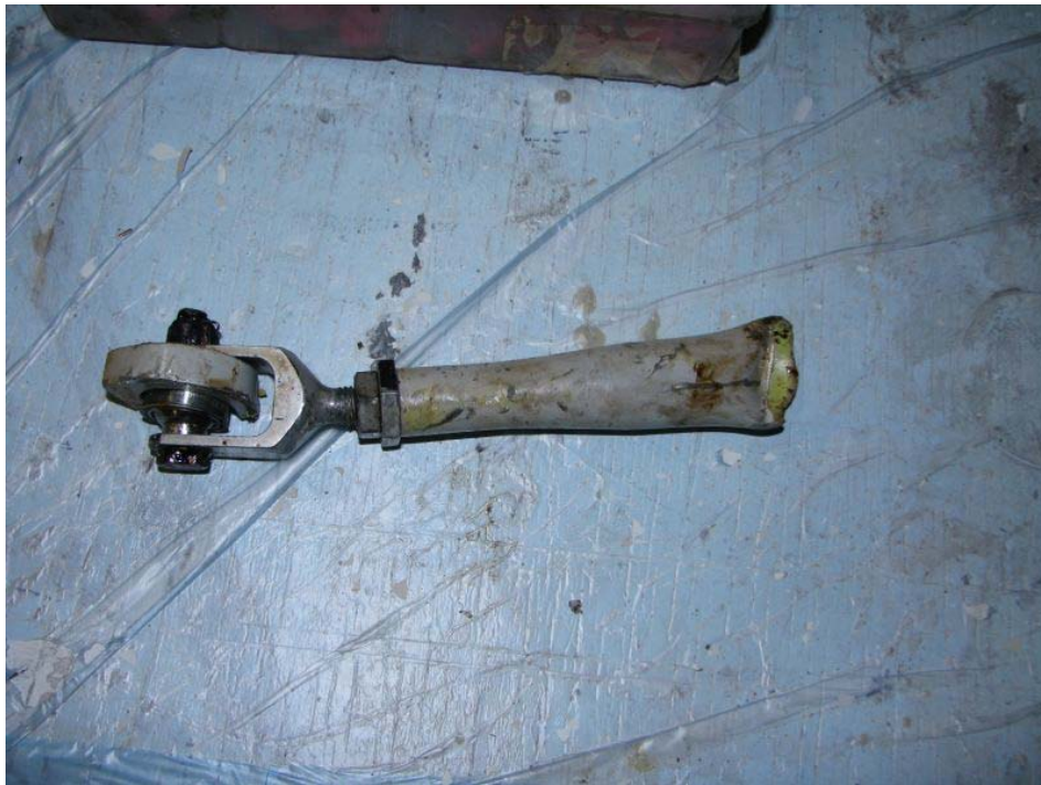
Photo 11 Bottom fractured section of White pitch change link with attached swashplate ear
