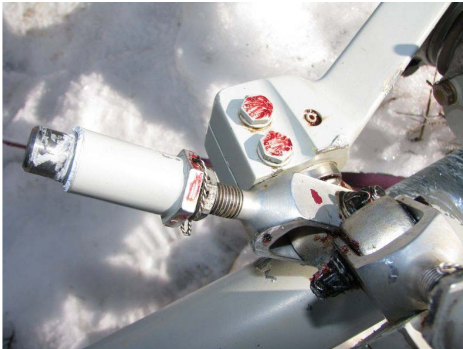
Photo 12 Top of Red pitch change link fractured consistent with overload near insert
