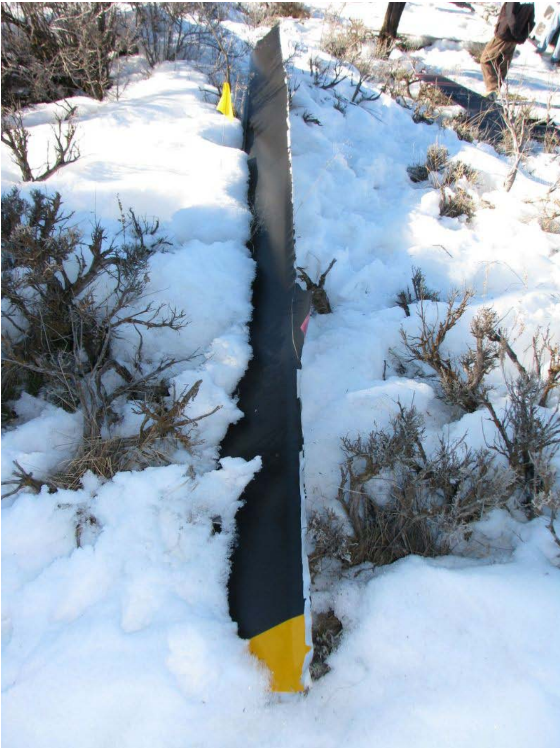
Photo 18 White main rotor blade outboard fractured section
