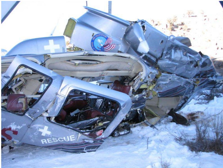
Photo 1 Crushing on left side of fuselage
