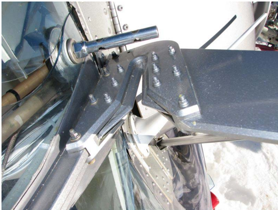
Photo 2 Upper wirestrike cutter showed no evidence of wire contact
