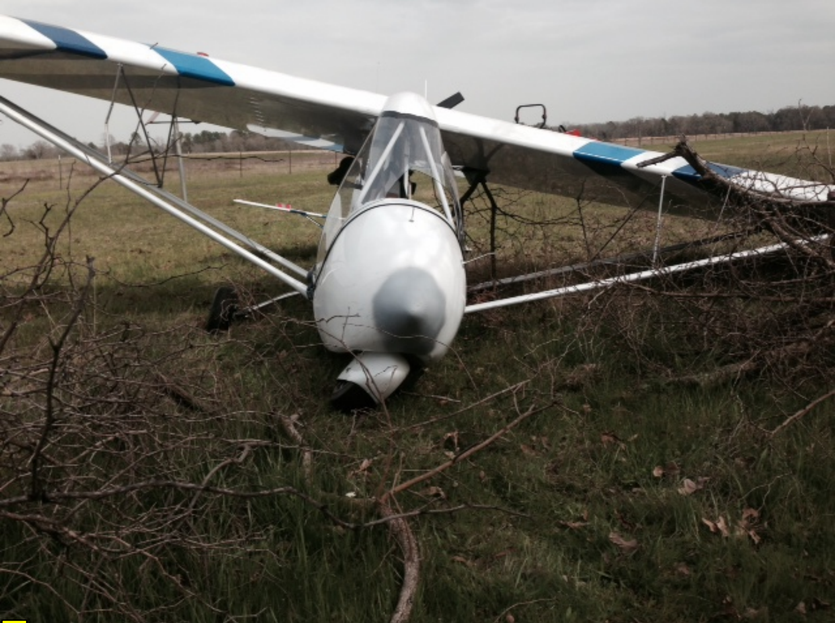
Photo 4. Collapsed Nosed and Left Main Landing Gears, Buckled Struts and Tree Branches in Left Wing
