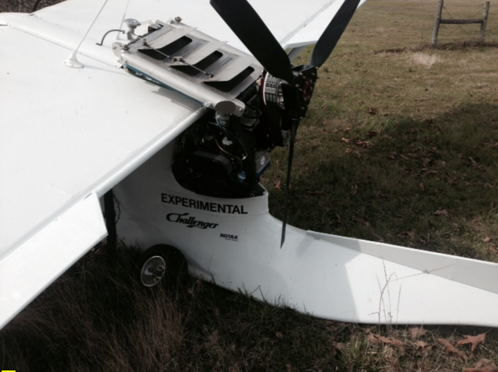
Photo 3. Collapsed Left Main Landing Gear and Buckled Fuselage
