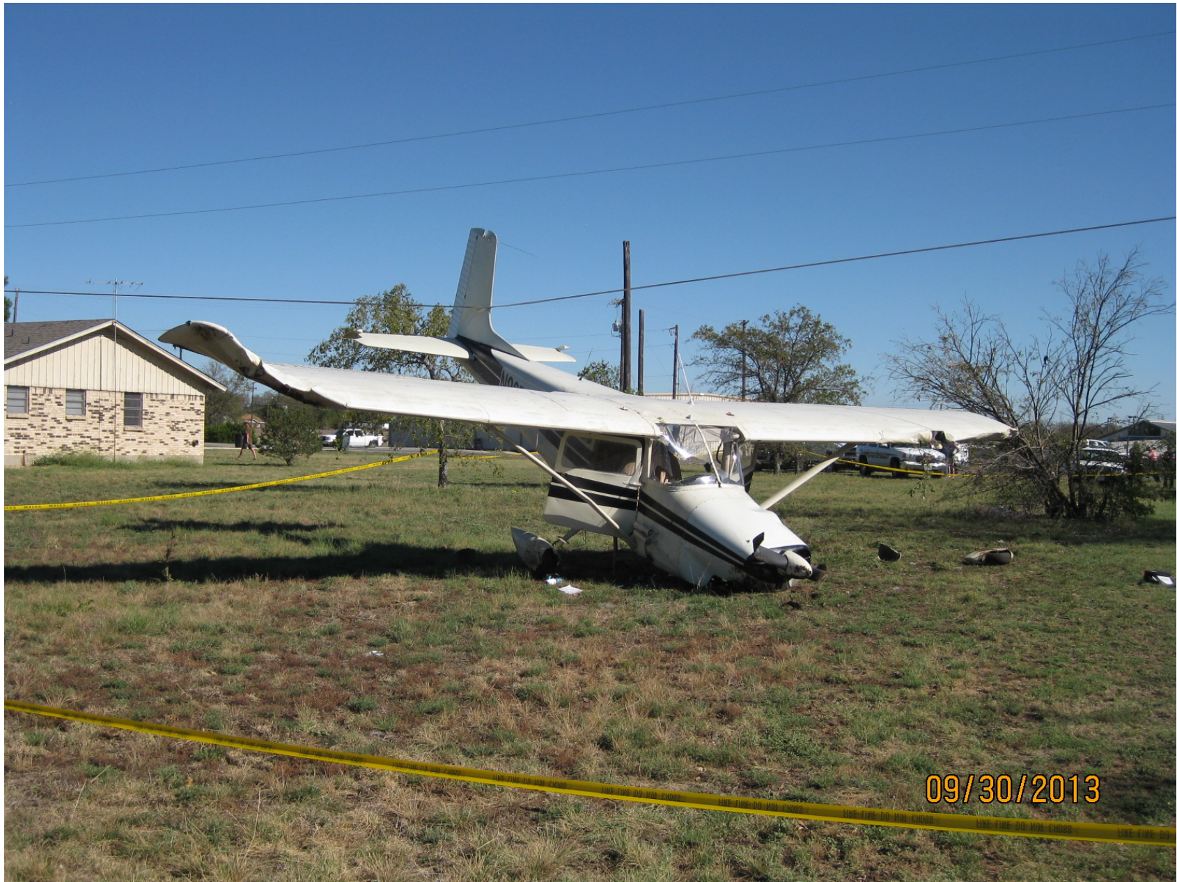
Photo 2 – Airplane viewed from front, nose gear collapsed, both wings damaged
