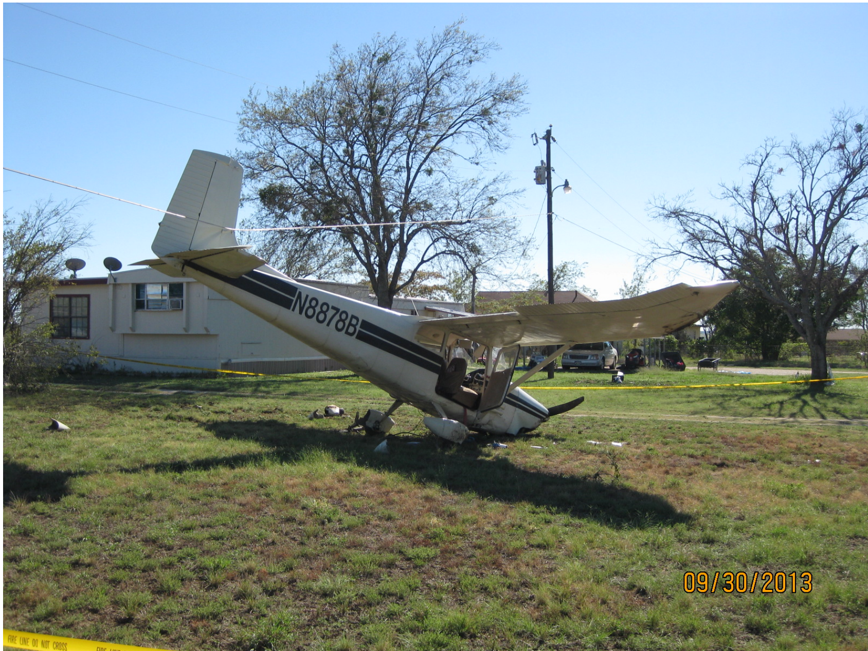
Photo 1 – Airplane in yard, viewed from right side, nose gear collapsed
