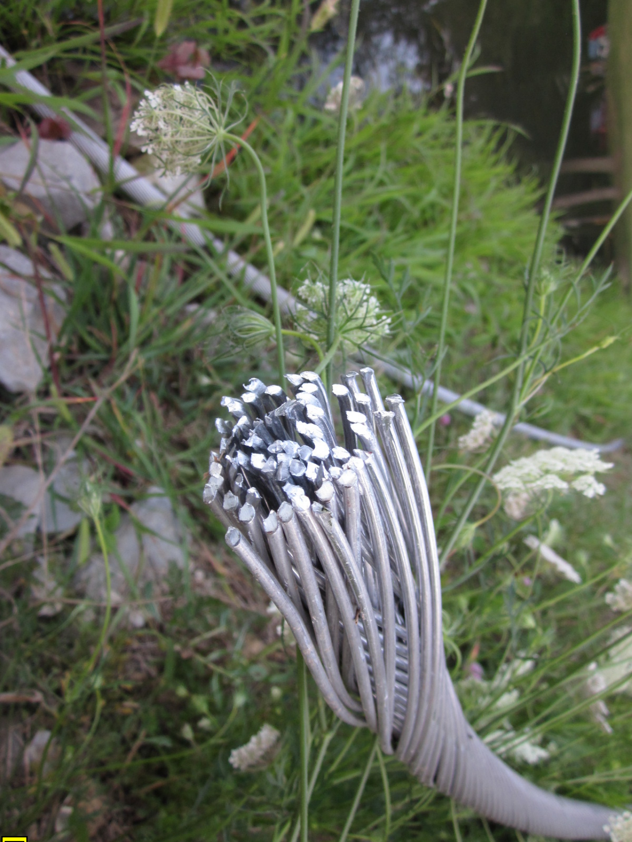
Photo 3: Severed power line
