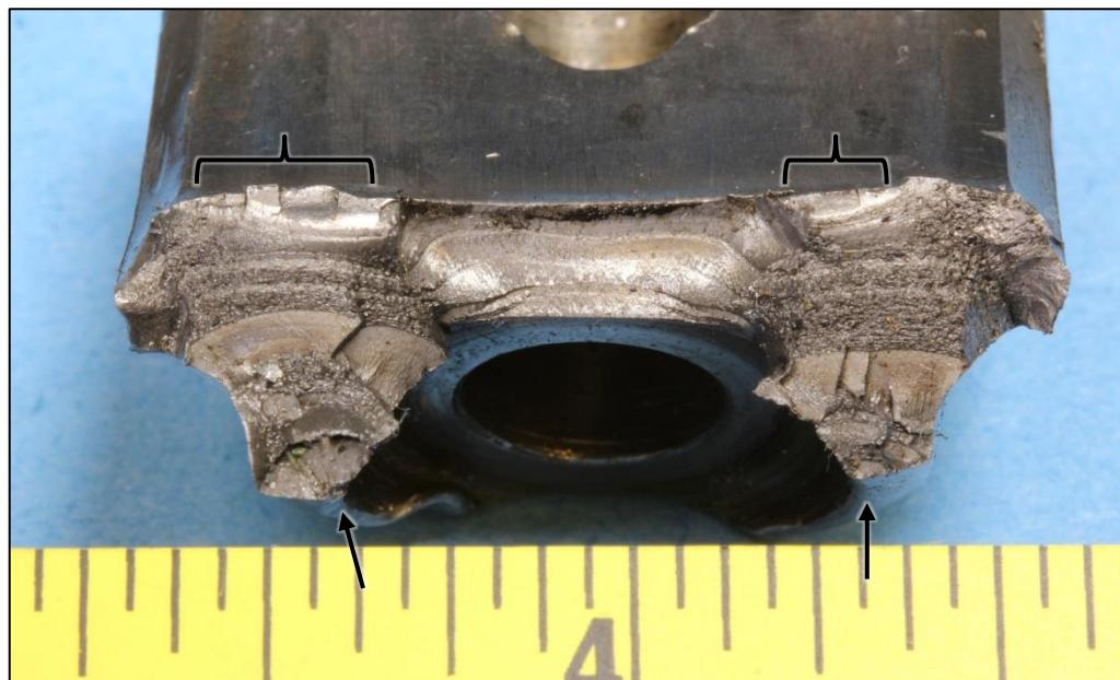
Figure 2. Overall view of a fracture surface on a strap piece from the number 2 connecting rod. Arrows and brackets indicate fatigue origin areas on opposite sides of the fracture surface.
