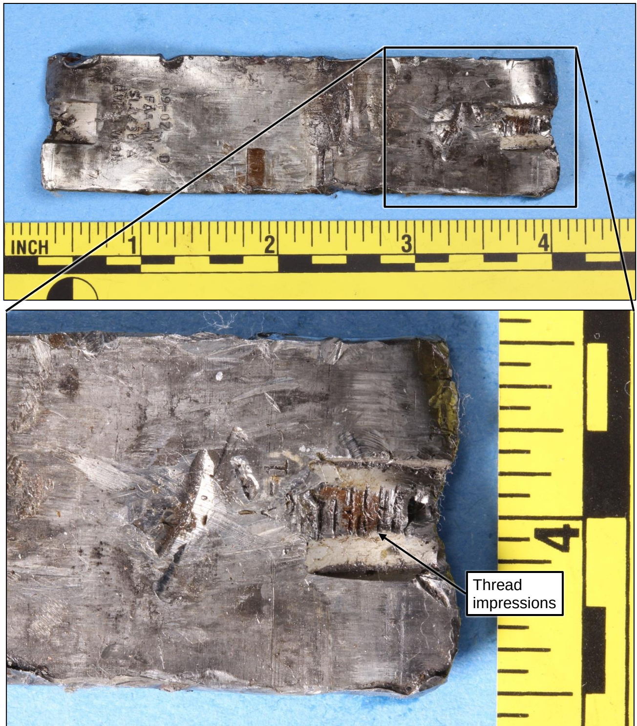
Figure 4. Views of the backside of one of the bearings showing thread impressions corresponding to contact with the threads of a connecting rod bolt.
