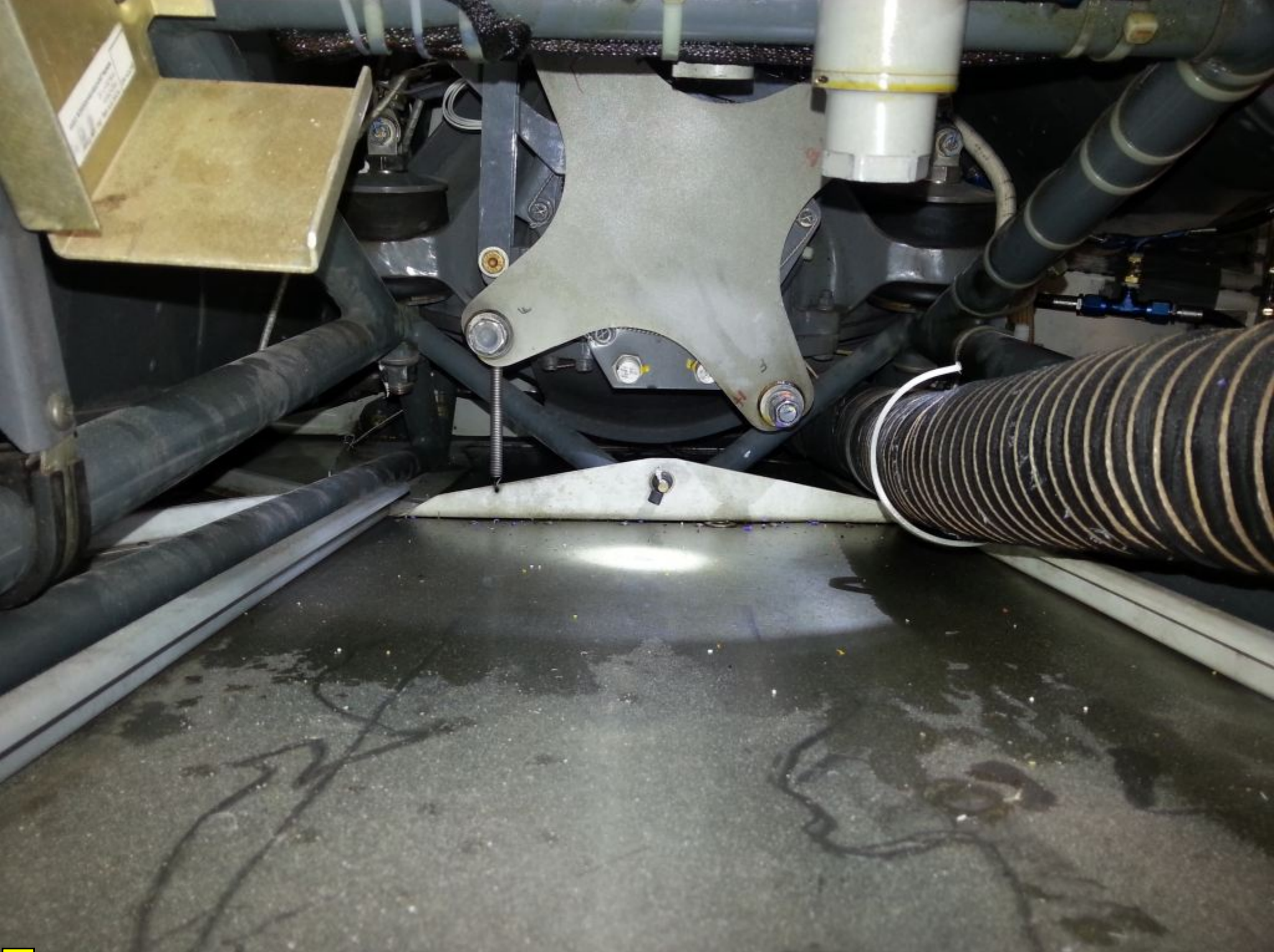
Photo 5 - The magnet was found affixed to a bolt just aft of the yoke, and a small dent was found on the horizontal firewall.
