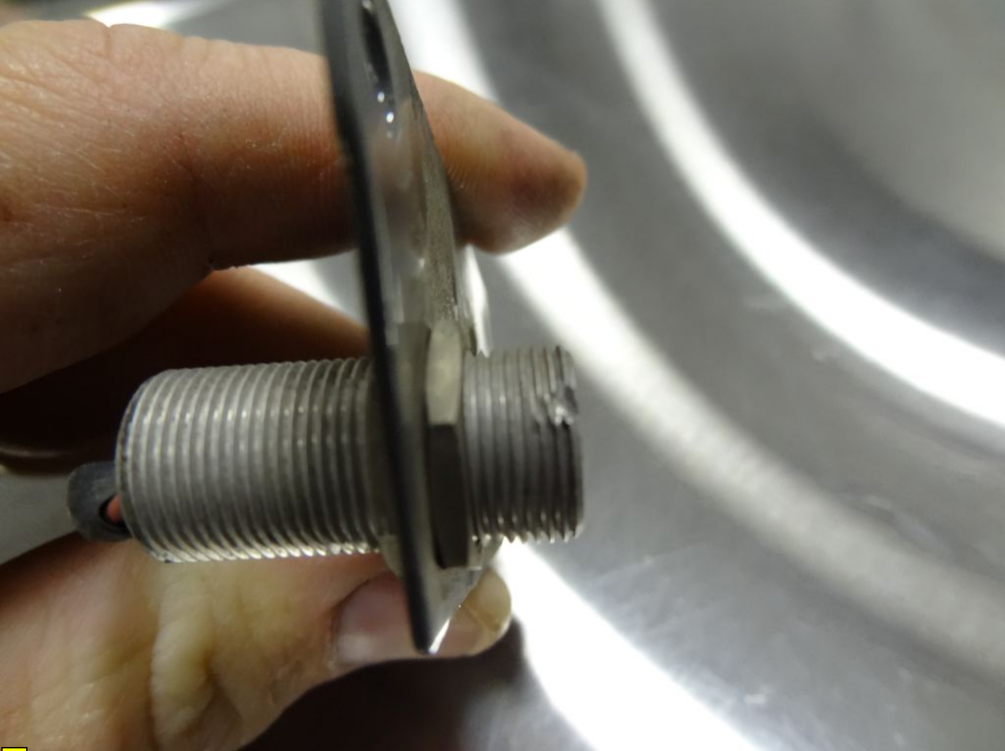
Photo 4 - Mechanical damage to the sensor, caused by the failed magnet. It was mounted oppsite the magnet.
