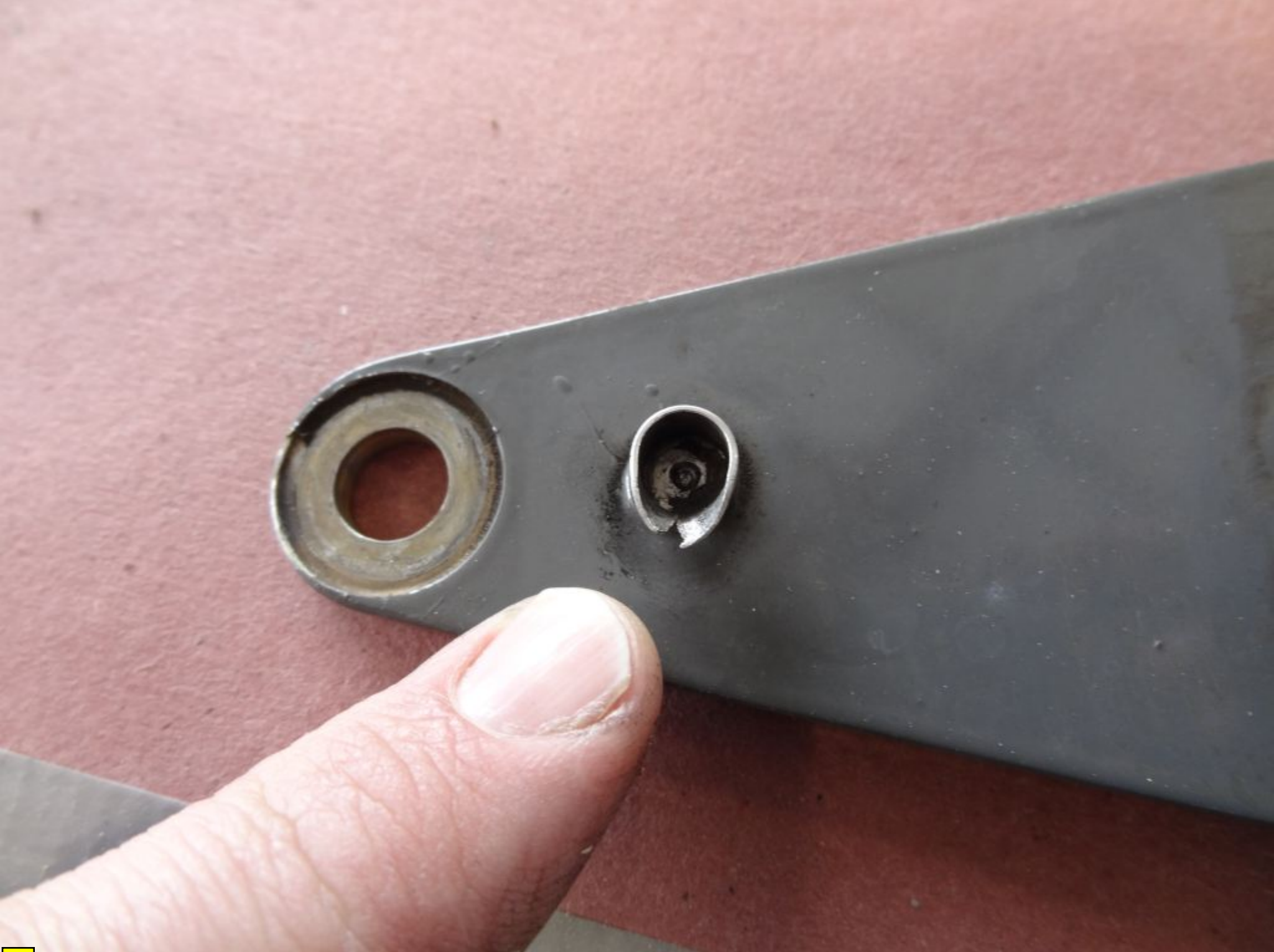
Photo 3 - Close-up view of the missing magnet.
