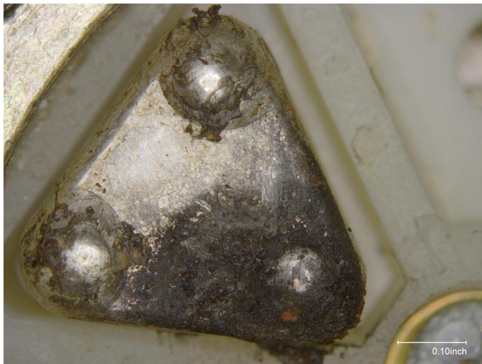
Figure 2. Photograph of residue on contact surface.
