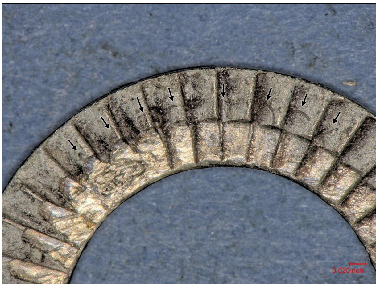
Figure 3. Close view of one of the washers showing the upper portions of characters consistent with NORD LOCK as indicated with arrows.
