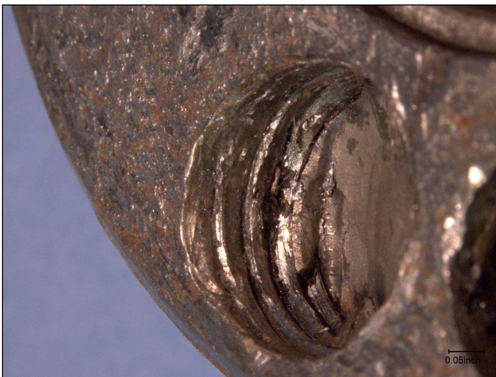
Figure 5. Close view of thread damage at bolt hole 4 (upper image) and 3 (lower image) on the crankshaft piece.
