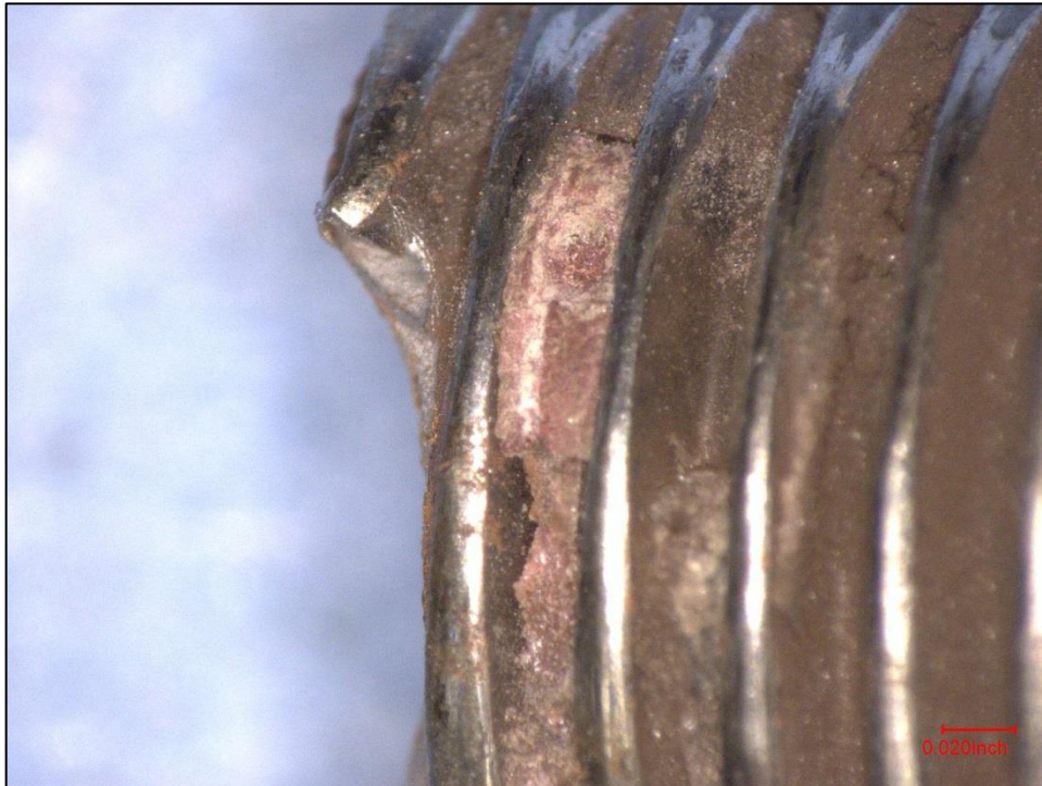
Figure 6. Red-colored thread lock observed in the threads of fractured attachment bolt number 6.
