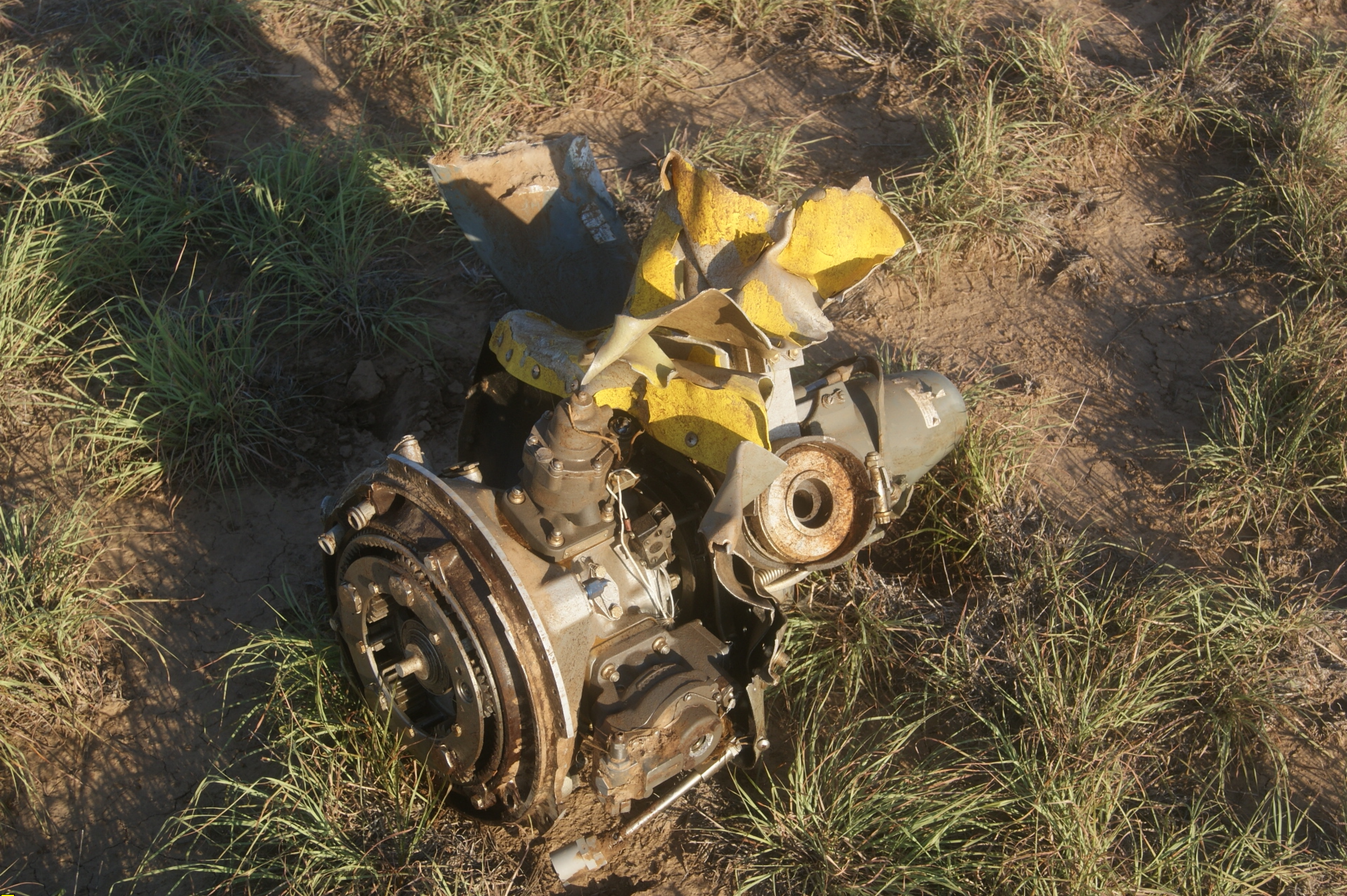
Photo 8 – Forward engine gearbox separated at A-frame with propeller hub attached and planetary gears visible.
