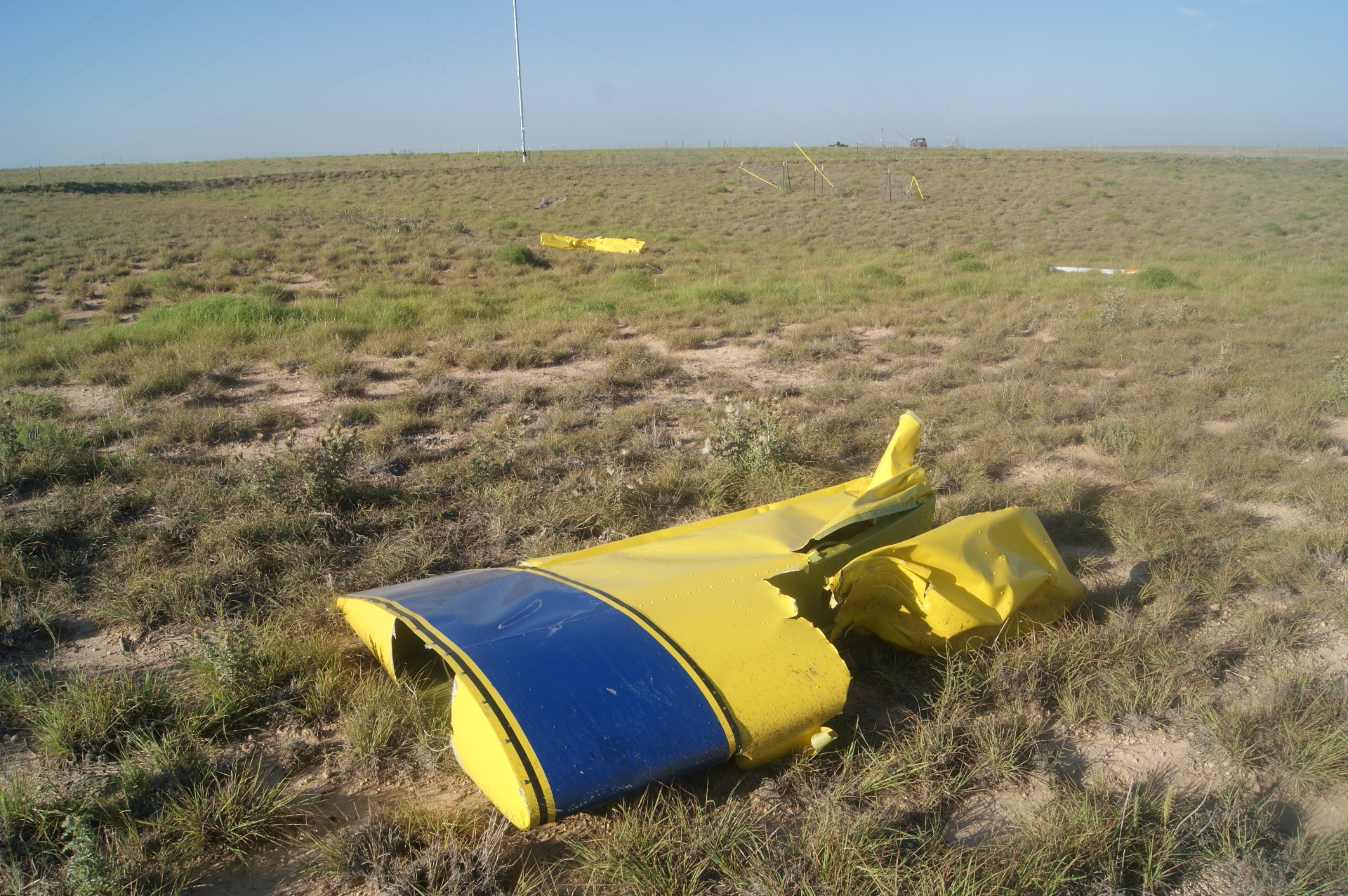
Photo 3 - Severed right wing with leading edge gouge. Right aileron and meteorological tower are in background.
